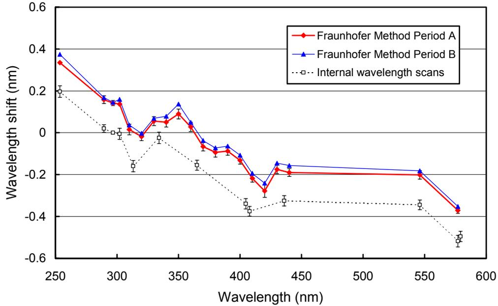
**Figure 5.1.7.** Monochromator non-linearity for the McMurdo 1999-2000 season. Lines: Correction functions calculated with the Fraunhofer-correlation method for Periods A and B. Broken line: Correction function calculated with the method that was historically applied. The offset difference between both methods is 0.14 nm. The error bars show the  $1\sigma$  standard deviation of the wavelength shift.
