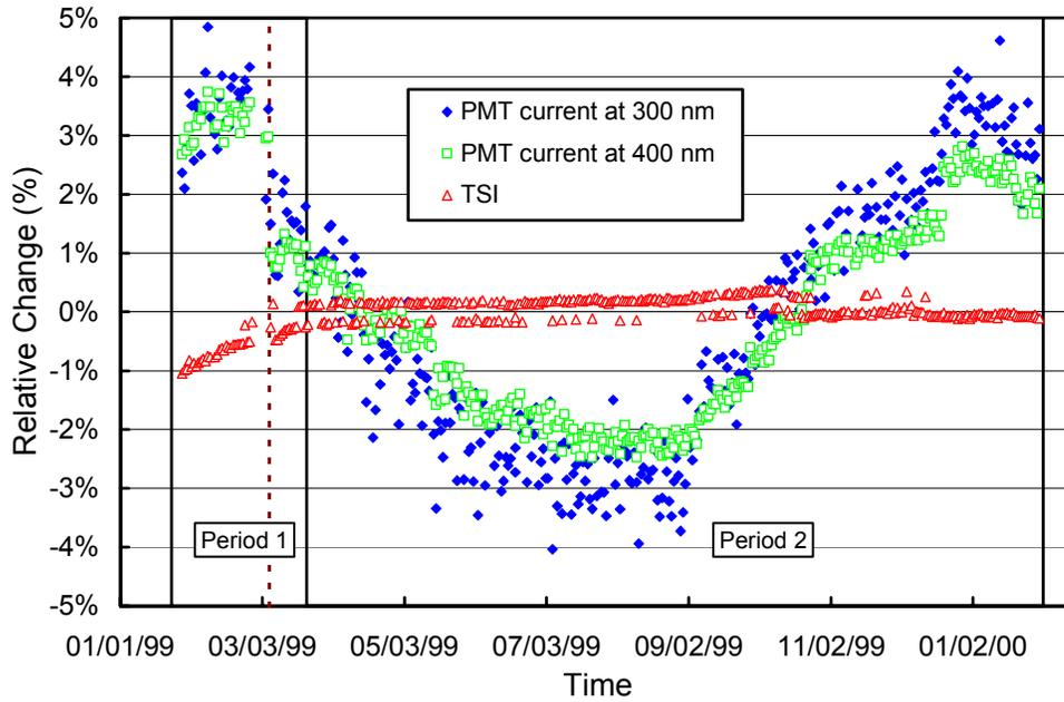
**Figure 5.1.3.** Time-series of PMT current at 300 and 400 nm, and TSI signal during measurements of the internal irradiance reference lamp during the McMurdo 1999-2000 season. The data is normalized to the average value of the whole season. The dashed line indicates the day when the wavelength correction table was changed.
