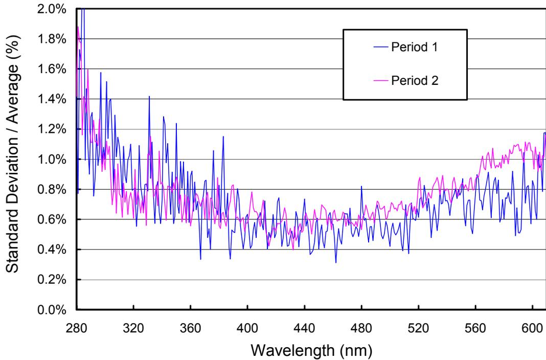
**Figure 5.1.5.** Ratio of standard deviation and average calculated from the absolute calibration scans measured during the McMurdo 1999-2000-season.
