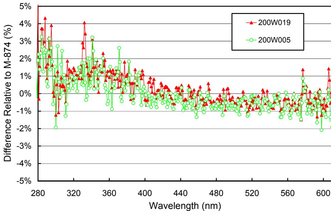
**Figure 5.1.2.** Comparison of McMurdo lamps 200W005 and 200W019 with the BSI traveling standard M-874 at the end of the season (1/31/00).
