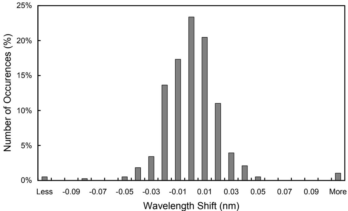
**Figure 5.1.6.** Differences in the measured position of the 296.73 nm mercury line between consecutive wavelength scans. The x-labels give the center wavelength shift for each column. The 0-nm histogram column covers the range  $-0.005$  to  $+0.005$  nm. “Less” means shifts smaller than  $-0.105$  nm; “more” means shifts larger than  $0.105$  nm.
