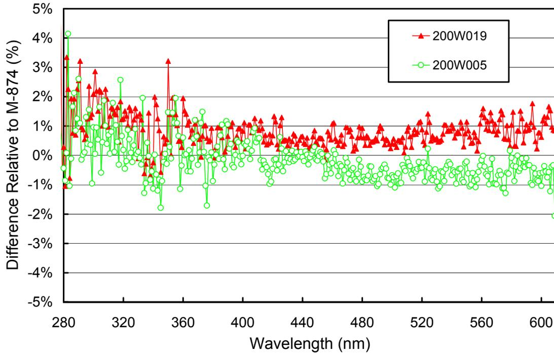
**Figure 5.1.1.** Comparison of McMurdo lamps 200W005 and 200W019 with the BSI traveling standard M-874 at the beginning of the season (1/24/99).
