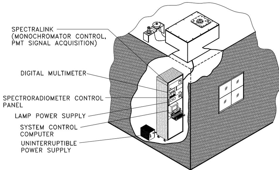
**Figure 2.4.** *Diagram of electronic components and computer. Access to the instrument mounted on the roof is typically provided above the installation.*
