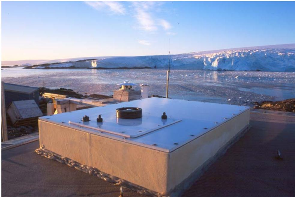
**Figure 2.2.** Top part of the SUV-100 spectroradiometer at the installation at Palmer Station. The irradiance collector is the black ring with the white Teflon<sup>®</sup> diffuser in the middle. At the left of the collector is a connector for the external calibration fixture.
