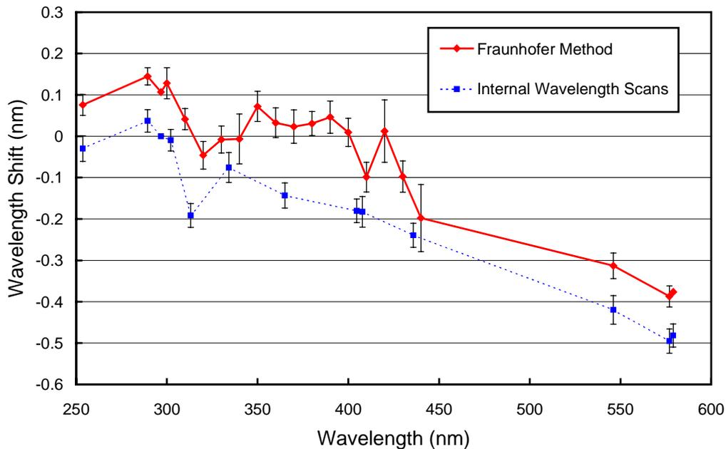
**Figure 5.5.6.** Monochromator non-linearity for the San Diego 1998-99 season. Solid line: Correction function calculated with the Fraunhofer-correlation method, applied to correct the San Diego Volume 8 data. Broken line: Correction function calculated with the method that was historically applied. The offset difference between both methods is 0.11 nm. The error bars show the  $1\sigma$  standard deviation of the wavelength shift for the season.
