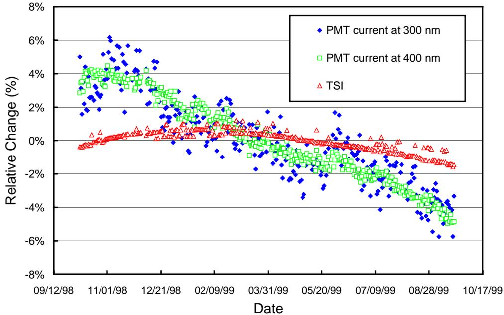
**Figure 5.5.3.** Time-series of PMT current at 300 and 400 nm, and TSI signal during measurements of the internal irradiance reference lamp during the San Diego 1998-99 season. The data is normalized to the average value of the whole season.
