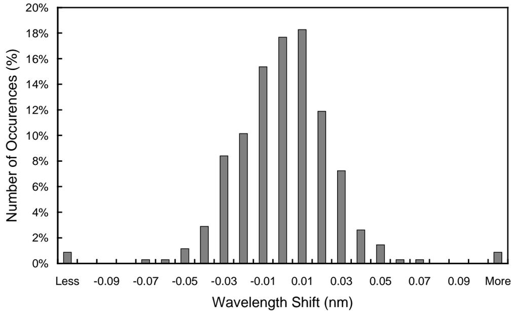
**Figure 5.5.5.** Differences in the measured position of the 296.73 nm mercury line between consecutive wavelength scans. The x-labels give the center wavelength shift for each column. The 0-nm histogram column covers the range -0.005 to +0.005 nm. “Less” means shifts smaller than -0.105 nm; “more” means shifts larger than 0.105 nm.
