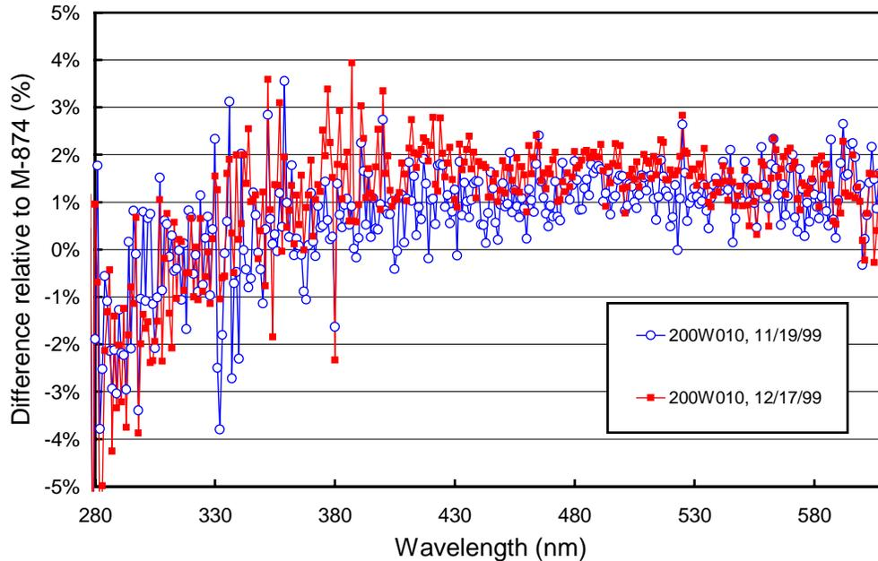
**Figure 5.5.2.** Comparison of standards 200W010 and M-874. The absolute scan with lamp M-874 was performed on 12/3/99. The good agreement of the two absolute scans with 200W010 conducted on 11/19/99 and 12/17/99 indicates that the system was very stable during this period. Hence, the comparison is valid, although the lamps were not operated on the same day, as it is usually done.
