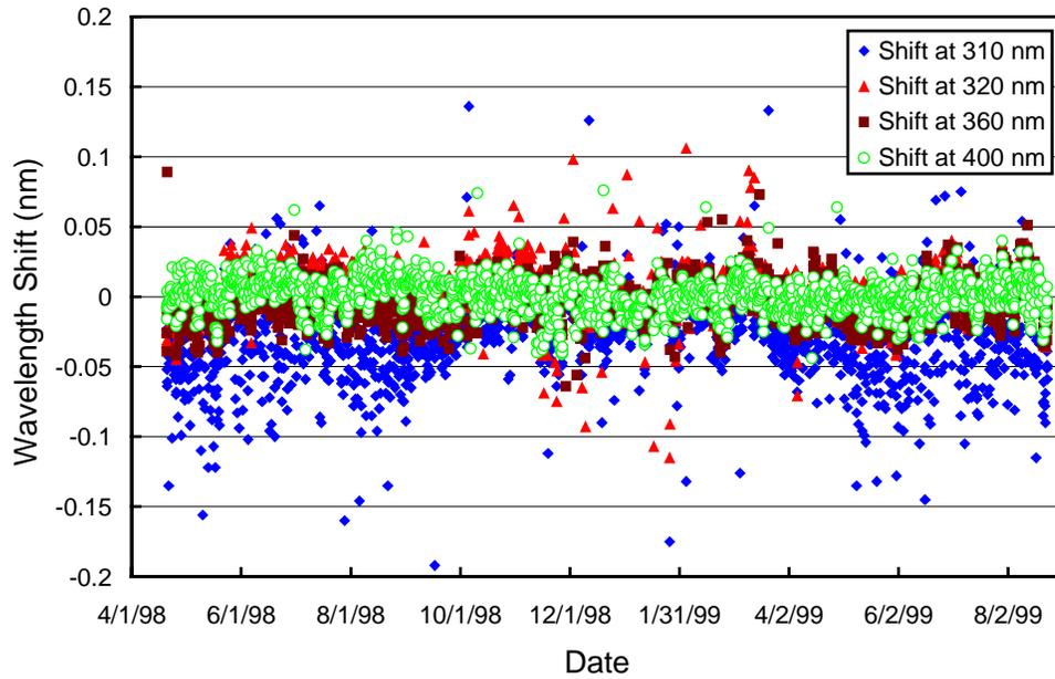
**Figure 5.4.10.** *Wavelength accuracy check of the final data at four wavelengths by means of Fraunhofer correlation. Measurements at four different times of the day have been evaluated for each day of the season.*
