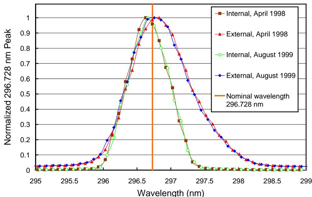
**Figure 5.4.11.** *The 296.73 mercury line as registered by the PMT from external and internal sources. The wavelength scale is the same as applied for solar measurements, i.e., it is based on a combination of internal scans and the Fraunhofer-correlation method. It is assumed that the wavelength registration of the monochromator did not shift between internal and external scans, which were close in time.*
