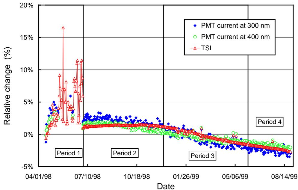
**Figure 5.4.4.** Time-series of PMT current at 300 and 400 nm and TSI signal during measurements of the response lamp during the Ushuaia 1998-99 season. The data is normalized to the average of Periods 2-4.
