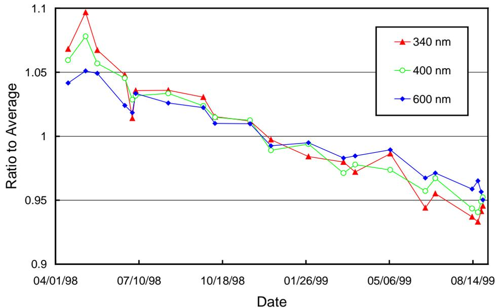
**Figure 5.4.5.** Temporal change of PMT current at several wavelengths during measurements of the site standard 200W008.
