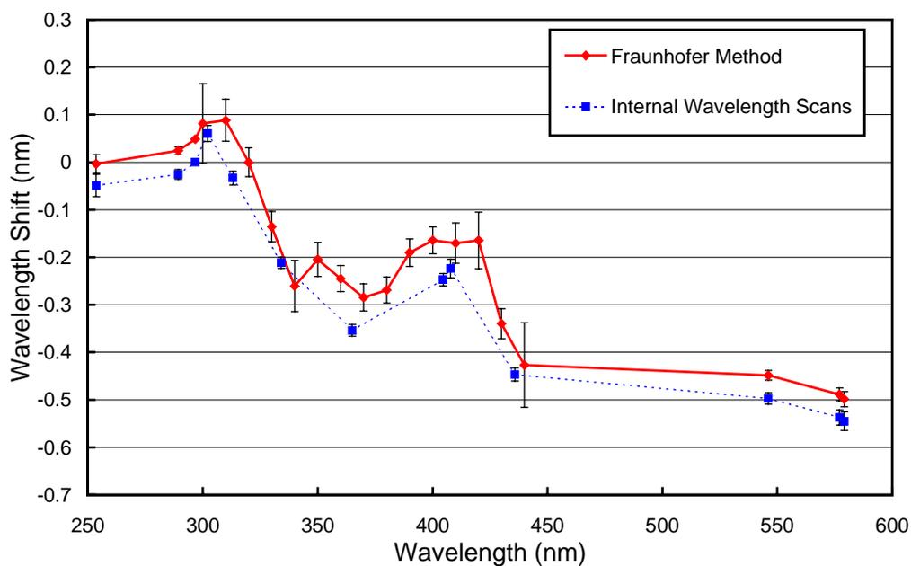
**Figure 5.4.9.** Monochromator non-linearity for the Ushuaia 1998-99 season. Heavy line: Correction function calculated with the Fraunhofer-correlation method, applied to correct the Ushuaia Volume 8 data. Thin broken line: Correction function calculated with the method that was historically applied. The offset difference between both methods is 0.08 nm. The error bars are the  $1\sigma$  standard deviation of the wavelength shift for the season.
