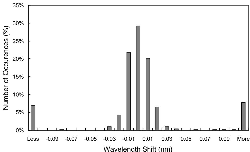
**Figure 5.4.8.** Differences in the measured position of the 296.73 nm mercury line between consecutive wavelength scans. The labels of the horizontal axis give the center wavelength shift for each column. The 0-nm histogram column covers the range from -0.005 to +0.005 nm. “Less” means shifts smaller than -0.105 nm; “more” means shifts larger than 0.105 nm.
