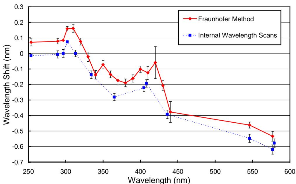
**Figure 5.3.6.** Monochromator non-linearity for the South Pole 1998-99 season. Thick line: Correction function calculated with the Fraunhofer-correlation method, applied to correct the South Pole Volume 8 data. Thin broken line: Correction function calculated with the method that was historically applied. The offset difference between both methods is 0.08 nm. The error bars show the  $1\sigma$  standard deviation of the wavelength shift for the season.
