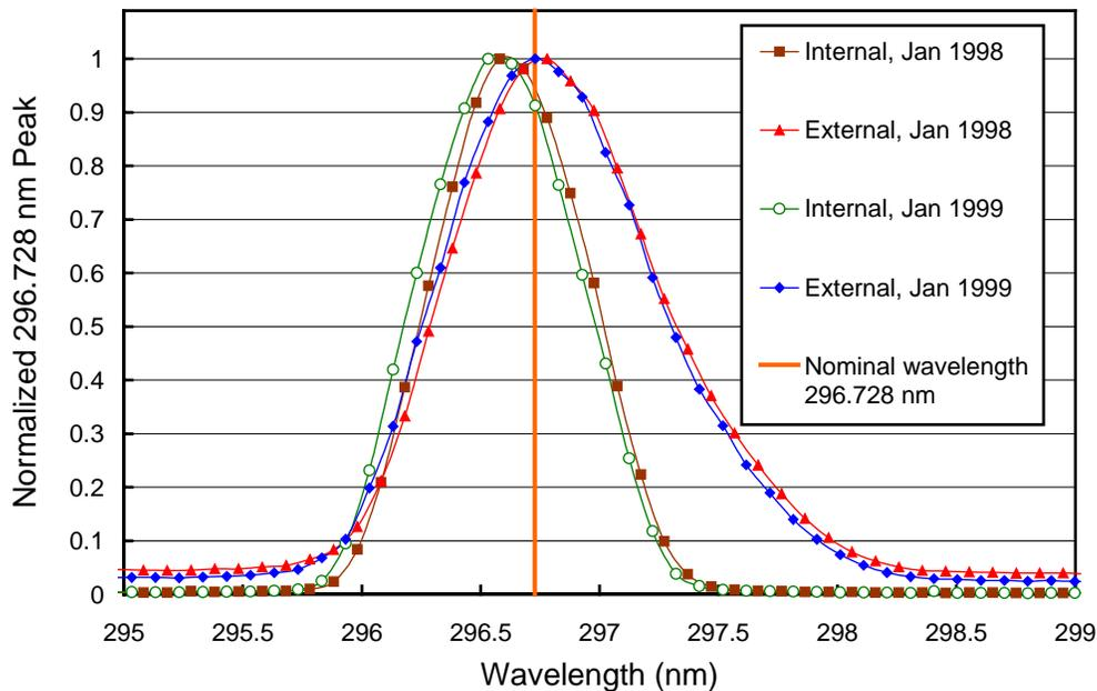
**Figure 5.3.8.** The 296.73 mercury line as registered by the PMT from external and internal sources. The wavelength scale is the same as applied for solar measurements, i.e., it is based on a combination of internal scans and the Fraunhofer-correlation method.
