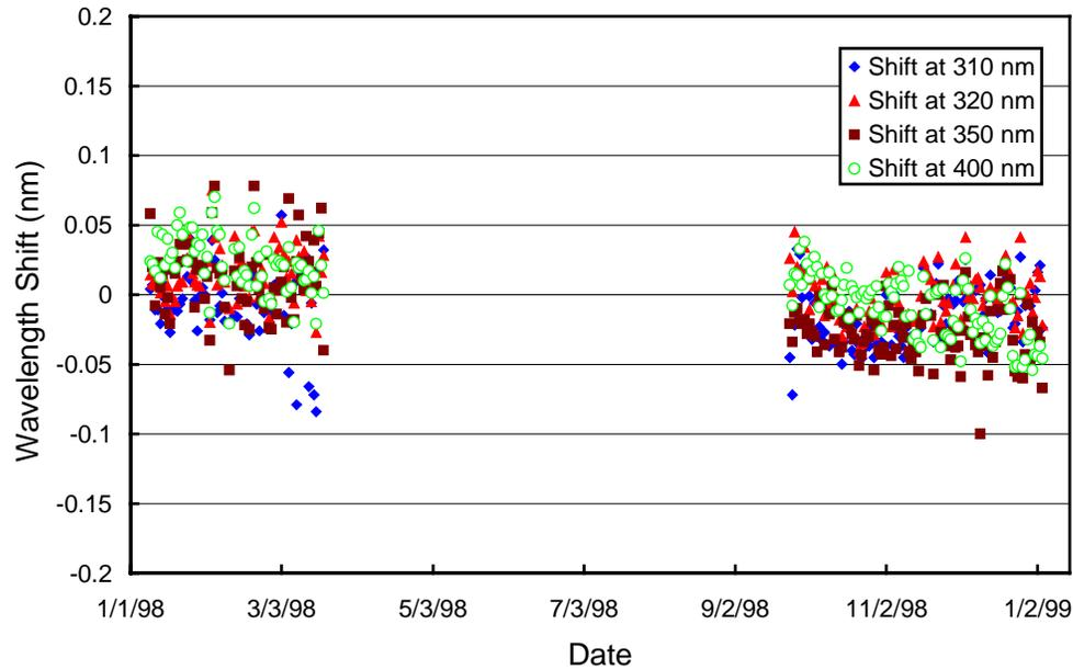
**Figure 5.3.7.** Wavelength accuracy check of the final data at four wavelengths by means of Fraunhofer correlation. The noontime measurement has been evaluated for each day of the season. No data exist during polar night from 3/21/98 – 9/23/98.
