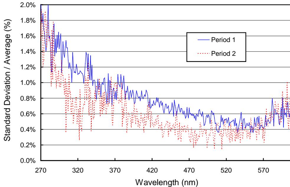
**Figure 5.2.4.** Ratio of standard deviation and average calculated from the absolute calibration scans of Periods 1 and 2.
