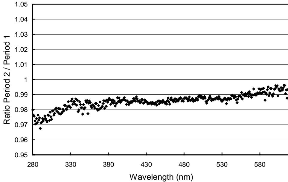
**Figure 5.2.5.** Ratio of irradiance assigned to the internal reference lamp in Period 2 and Period 1.
