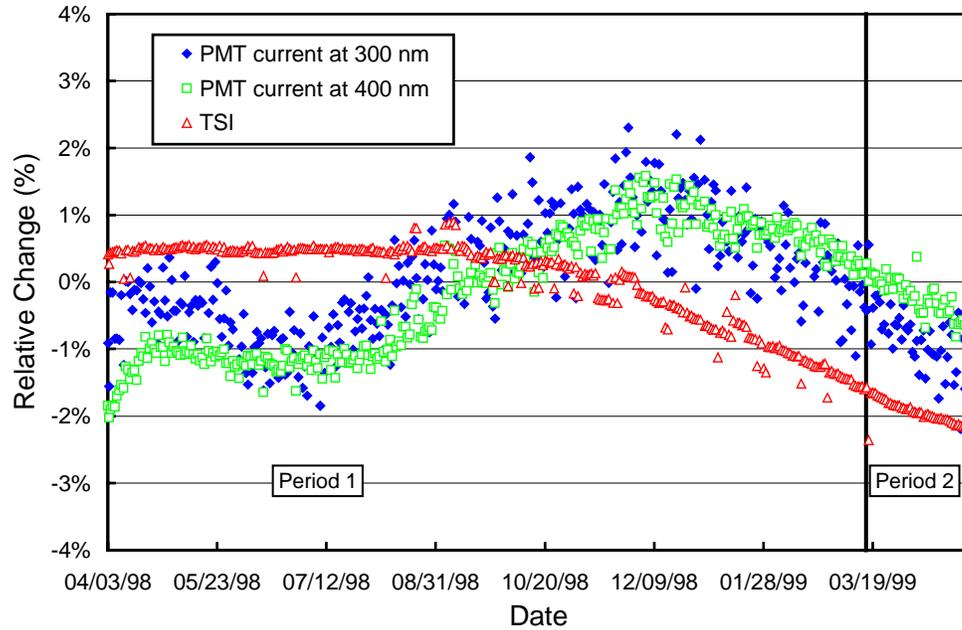
**Figure 5.2.3.** Time-series of PMT current at 300 and 400 nm and TSI signal during measurements of the response lamp during the Palmer 1998-99 season. The data is normalized to the average of both periods.
