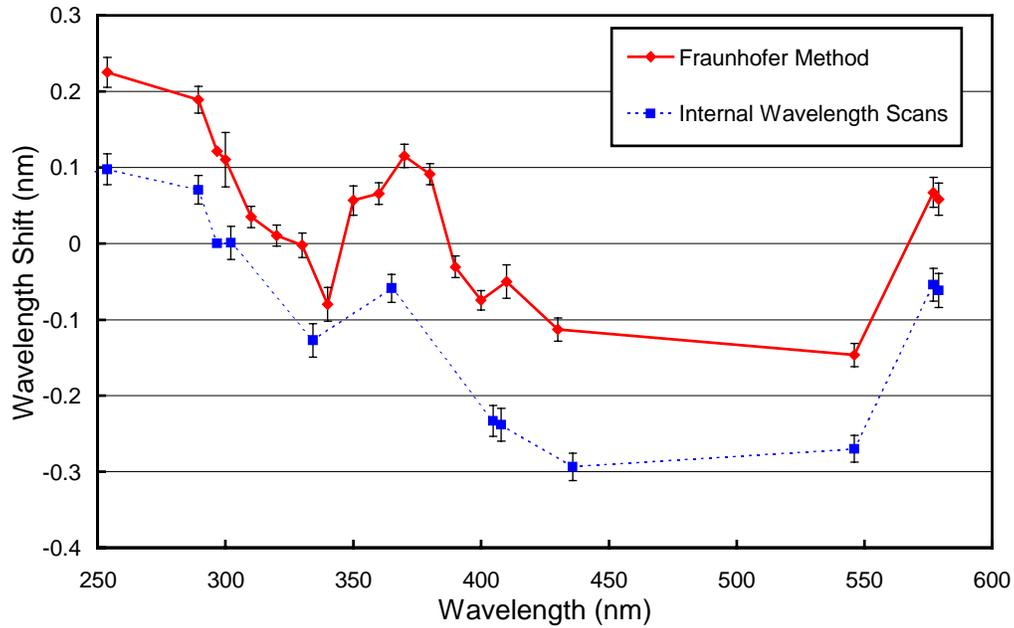
**Figure 5.2.7.** Monochromator non-linearity for the Palmer 1998-99 season. Thick line: Correction function calculated with the Fraunhofer-correlation method, applied to correct the Palmer Volume 8 data. Thin broken line: Correction function calculated with the method that was historically applied. The offset difference between both methods is 0.12 nm. The error bars show the  $1\sigma$  standard deviation of the wavelength shift for the season.
