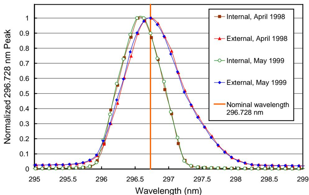
**Figure 5.2.9.** The 296.73 mercury line as registered by the PMT from external and internal sources. The wavelength scale is the same as applied for solar measurements, i.e., it is based on a combination of internal scans and the Fraunhofer-correlation method. It is assumed that the wavelength registration of the monochromator did not shift between internal and external scans, which were close in time.
