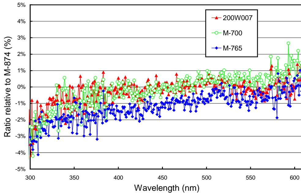
**Figure 5.2.2.** Comparison of Palmer lamps 200W007, M-700, and M-765 with the BSI traveling standard M-874 at the beginning of the season (day 4/2/98).
