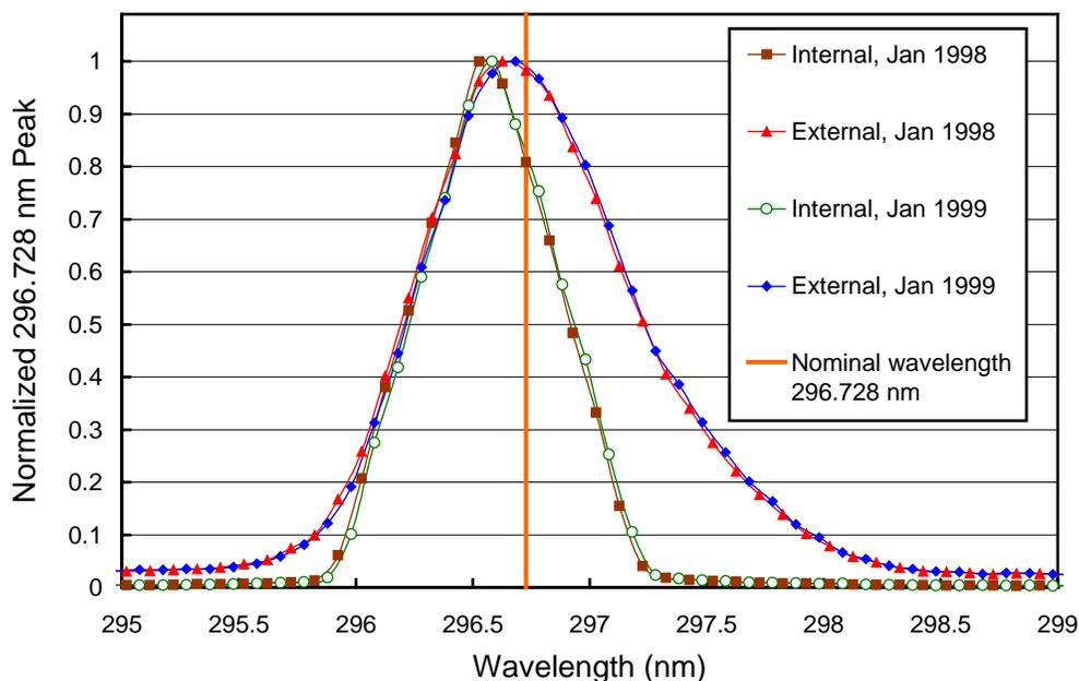
**Figure 5.1.8** The 296.73 mercury line as registered by the PMT from external and internal sources. The wavelength scale is the same as applied for solar measurements, i.e., it is based on a combination of internal scans and the Fraunhofer-correlation method. It is assumed that the wavelength registration of the monochromator did not shift between internal and external scans, which were close in time.
