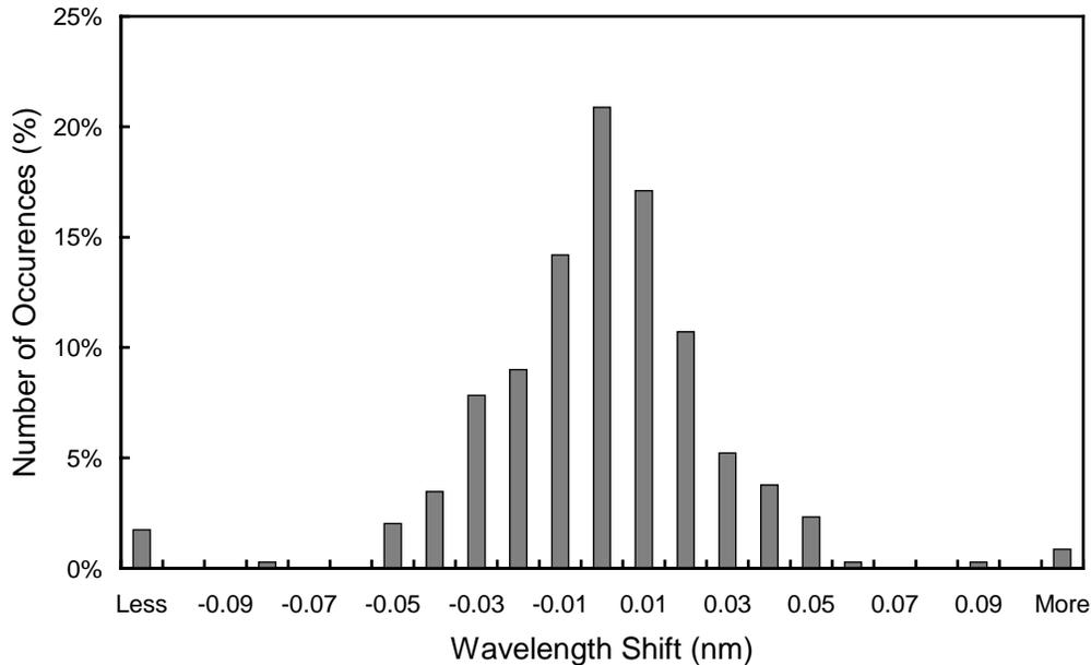
**Figure 5.1.5.** Differences in the measured position of the 296.73 nm mercury line between consecutive wavelength scans. The x-labels give the center wavelength shift for each column. The 0-nm histogram column covers the range -0.005 to +0.005 nm. “Less” means shifts smaller than -0.105 nm; “more” means shifts larger than 0.105 nm.
