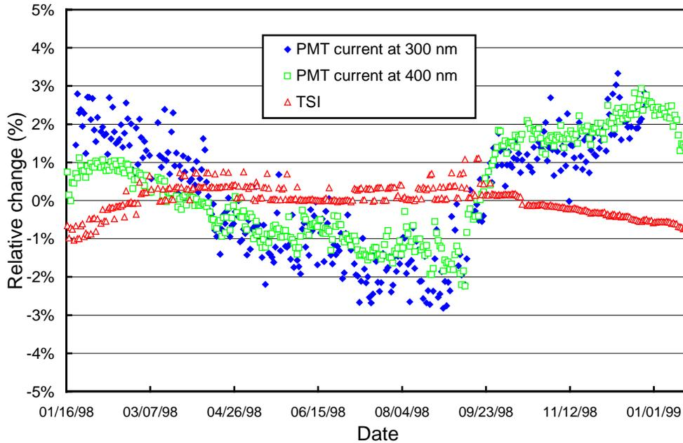
**Figure 5.1.3.** Time-series of PMT current at 300 and 400 nm, and TSI signal during measurements of the internal irradiance reference lamp during the McMurdo 1998-99 season. The data is normalized to the average value of the whole season.
