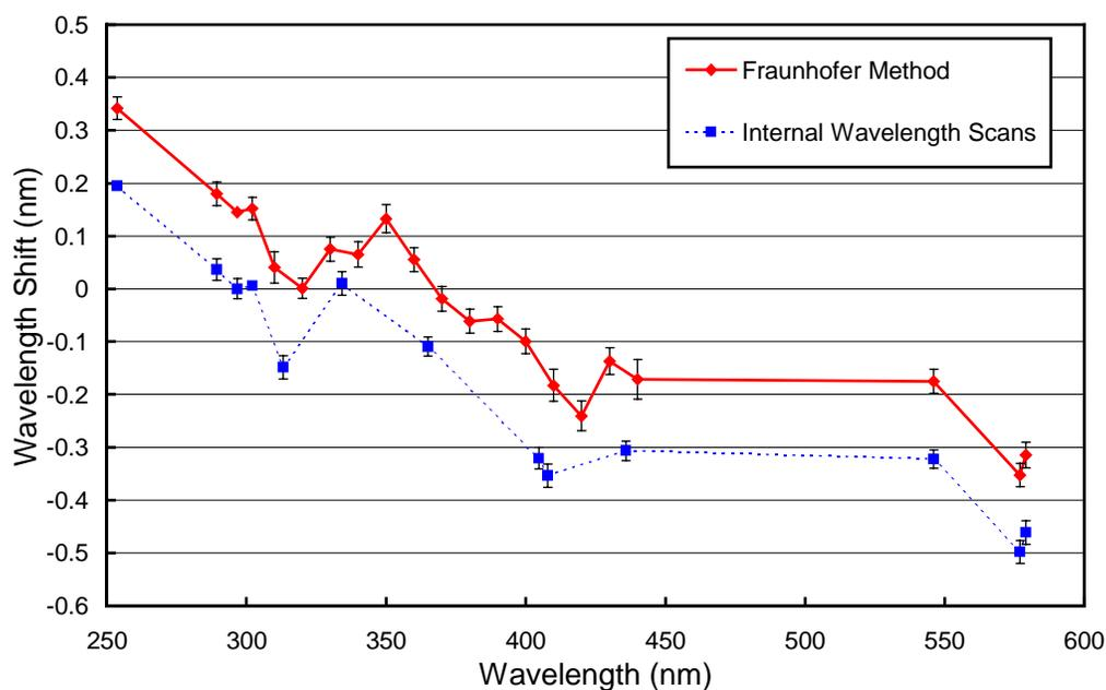
**Figure 5.1.6.** Monochromator non-linearity for the McMurdo 1998-99 season. Line: Correction function calculated with the Fraunhofer-correlation method, applied to correct the McMurdo Volume 8 data. Broken line: Correction function calculated with the method that was historically applied. The offset difference between both methods is 0.14 nm. The error bars show the  $1\sigma$  standard deviation of the wavelength shift for the season.
