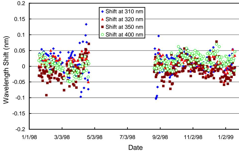
**Figure 5.1.7.** Check of the wavelength accuracy of the final data at four wavelengths by means of Fraunhofer correlation. The noontime measurement has been evaluated for each day of the season. No correlation data is available during the polar night.
