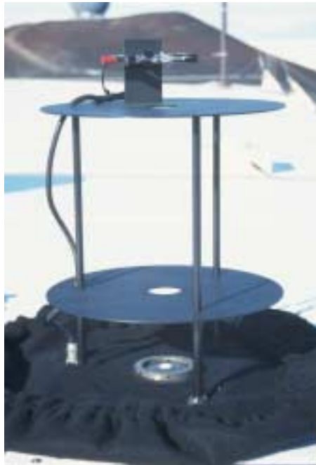
Figure 2.7. Calibration stand with the 200-Watt lamp mounted on top of the. The lamp power is connected to the roofbox immediately below the fixture. Baffles limit stray light. During operation, an internally-blackened barrel covers this fixture.
