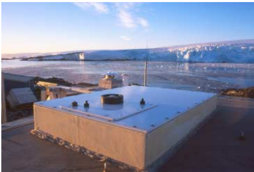
Figure 2.2. Top part of the SUV-100 spectroradiometer at the installation at Palmer Station. The irradiance collector is the black ring with the white Teflon ® diffuser in the middle. At the left of the collector is a connector for the external calibration fixture.
