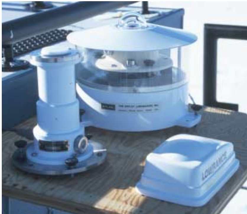
Figure 2.5. Eppley radiometers and GPS receiver. The PSP is shown in the background and is equipped with a ventilator that continuously blows air over the instrument case and its dome, keeping the hemispheres clean from frost and snow buildup. The TUVR radiometer is on the left; the GPS receiver is on the right.
