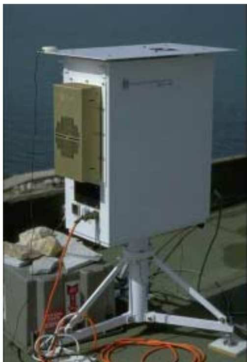
Figure 2.10. SUV-150 spectroradiometer at the SUSPEN intercomparison campaign held in Nea Michaniona, Greece in July 1997.
