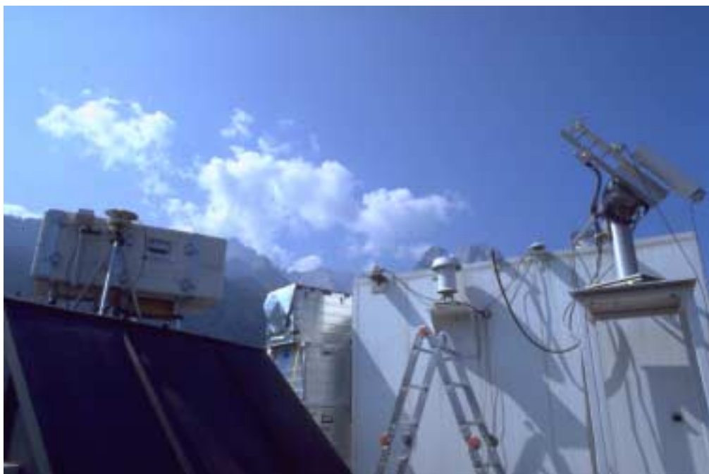
Figure 2.8. Instruments at an international intercomparison of UV spectroradiometers organized at the Fraunhofer Institute for Atmospheric Environmental Research (IFU), located in Garmisch-Partenkirchen, Germany. The portable SUV-100 is the instrument on the left. An Eppley PSP radiometer is placed on a tripod in front of the instrument. The stationary IFU spectroradiometer is located in the container on the right side. The apparatus to the far right is the suntracker of this instrument. Mountains of the Alps can be seen in the background.
