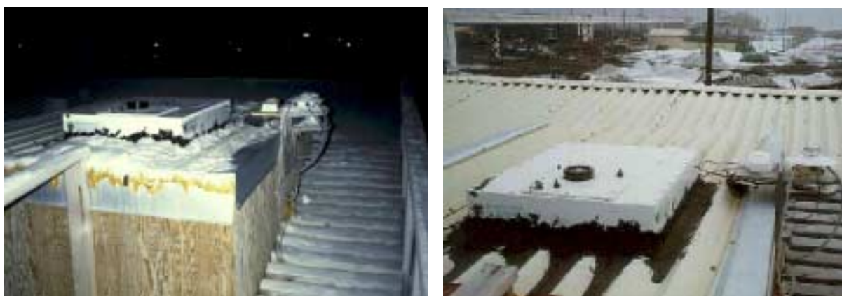
Figure 5.6.1. Roof installation at Barrow during the polar night (left). Note ice buildup on auxiliary sensors (right), and that the collector of the SUV-100, which is heated, remains free of snow, frost, and ice. Same installation during the day (right).
