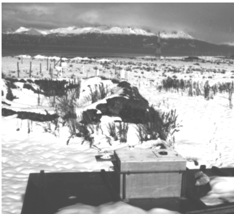
Figure 5.5.1. Roof box portion of the spectroradiometer installed in the roof of the CADIC facility in Ushuaia.
