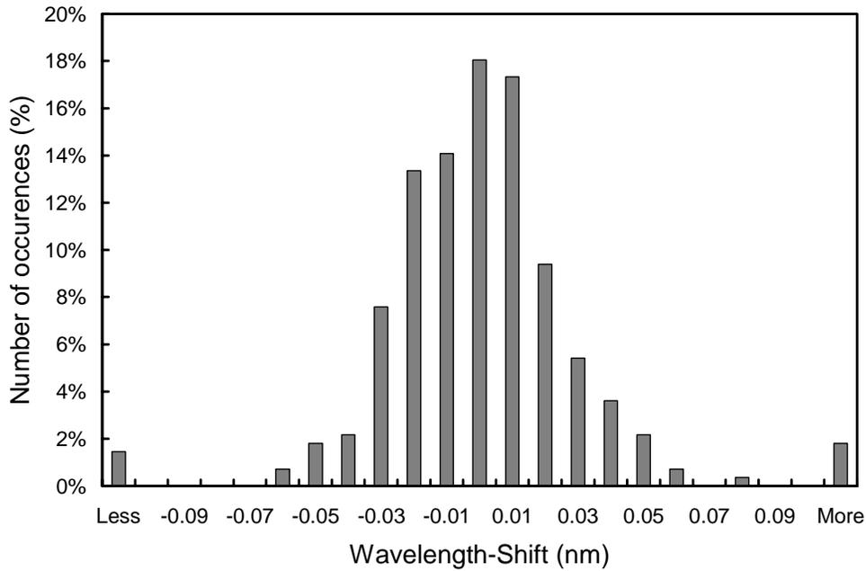
**Figure 5.4.5.** Differences in the measured position of the 296.72 nm Mercury line between consecutive wavelength scans. The x-labels give the center wavelength shift for each column. Thus the 0-nm histogram column covers the range -0.005 to +0.005 nm. “Less” means shifts smaller than -0.105 nm; “more” means shifts larger than 0.105 nm.
