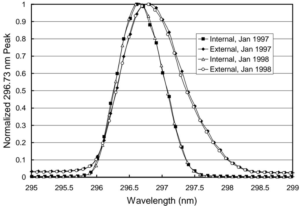
*Figure 5.4.8. The 296.73 mercury line as registered by the PMT from external and internal sources. For this plot, the wavelength calibration is based on the internal scans and it was assumed that the wavelength registration of the monochromator did not shift between internal and external scans, which were close in time.*
