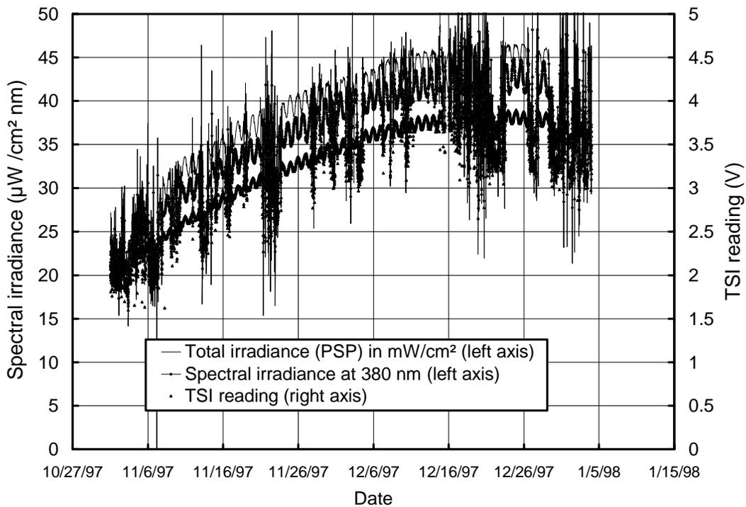
Figure 5.4.16. Comparison of total irradiance measured by the PSP (highest curve), spectral irradiance at 380 nm (middle curve), and TSI reading (lowest curve).
