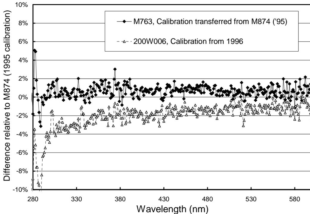
**Figure 5.4.14.** Season opening calibrations; comparison of the South Pole lamps M-763 and 200W006 with the traveling standard M-874 at the beginning of the season (1/27/97). The calibration of M-874 was established by Optronic Laboratories in 1998. The calibration of M-763 was transferred from M-874 and 200W006 was calibrated by Optronic Laboratories in 1996.
