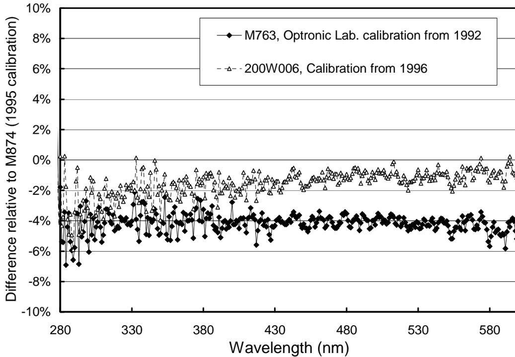
*Figure 5.4.13. Same as previous figure, except the calibration of M-763, which was established by Optronic Laboratories in 1992 rather than derived by transfer from M-874.*
