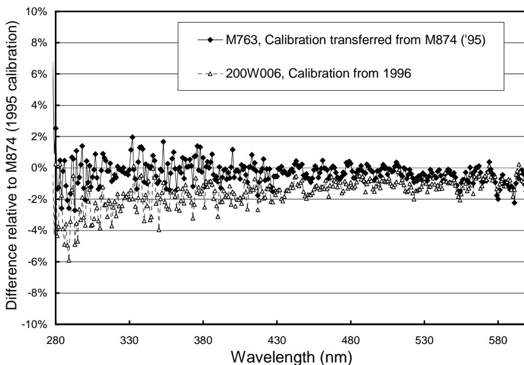
**Figure 5.4.12.** Season closing calibrations; Comparison of the South Pole lamps M-763 and 200W006 with the traveling standard M-874 at the end of the season (1/4/98). Optronic Laboratories established the calibration of M-874 in 1995. The calibration of M-763 was transferred from M-874, and Optronic Laboratories calibrated 200W006 in 1996.
