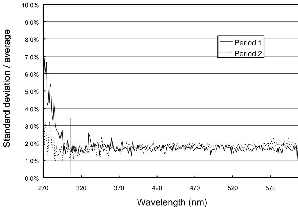
**Figure 5.4.10.** Ratio of standard deviation and average calculated from the absolute calibration scans of Periods 1 and 2. The vertical line marks 305 nm, which is the cut-off wavelength of Period 1 data.
