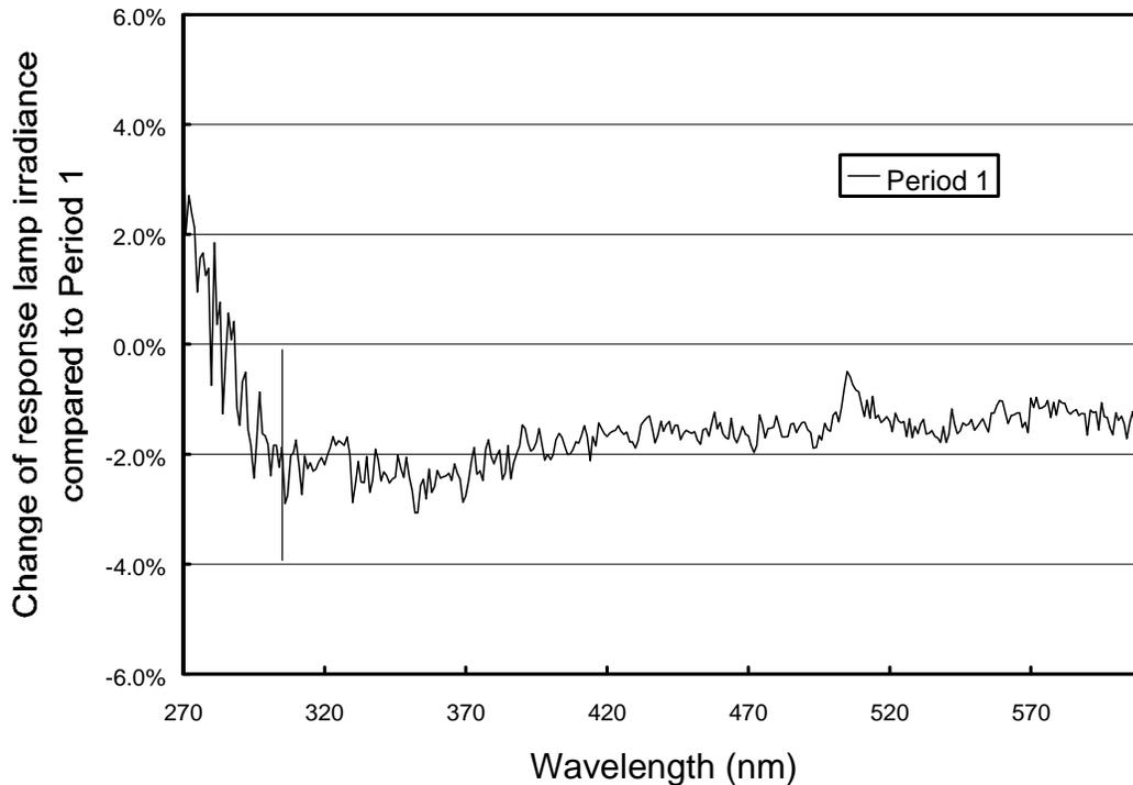
**Figure 5.4.11.** Change of the response lamp's "mean irradiance" between Periods 1 and 2. The vertical line marks 305 nm, which is the cut-off wavelength of Period 1 data.
