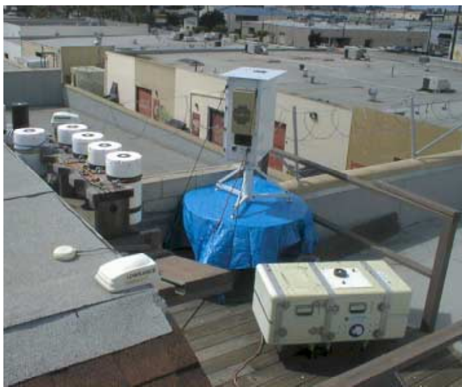
Figure 5.1.1. Test platform at Biospherical Instruments. SUV-100 installation (not shown) is in the roof seen to the left. Instruments shown here include the SUV-150 (top) and the portable SUV-100 (right foreground). On the edge of the roof in the foreground are two GPS receivers used for timekeeping, and at the left are several GUV and PUV radiometers also used in UV monitoring programs.
