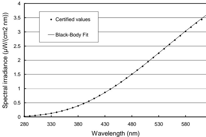
**Figure 3.20.** Spectral Irradiance of the San Diego site standard 200W010. The dots are the values from the lamp's certificate provided by Optronics Laboratories. The line through these points is the Black-Body fit.
