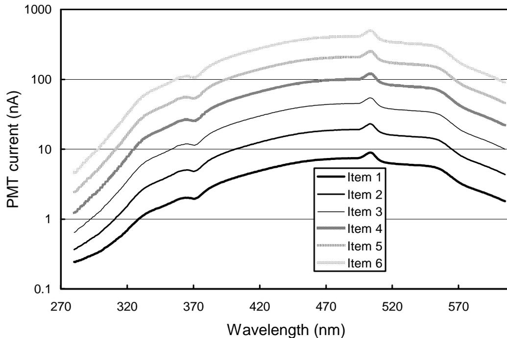
*Figure 3.4. Typical Response scan. Maximum PMT current may reach 1000 nA when the system is operated at peak sensitivity. The PMT dark current was not subtracted.*
