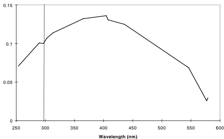
**Figure 3.15.** Typical difference between the monochromator corrections based on external and internal mercury scans. The vertical line emphasizes the difference at 296.73 nm.
