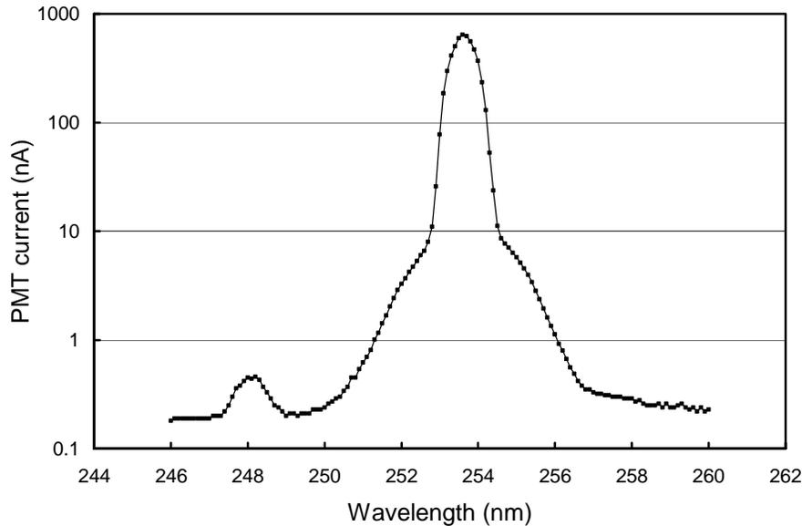
**Figure 3.5.** Wavelength scan in the vicinity of the Mercury peak at 253.65 nm. Blocks indicate the individual measurements. No dark value has been subtracted, and the data has not been corrected for the monochromator offset. The small peak at 248 nm is from a weaker Mercury line.
