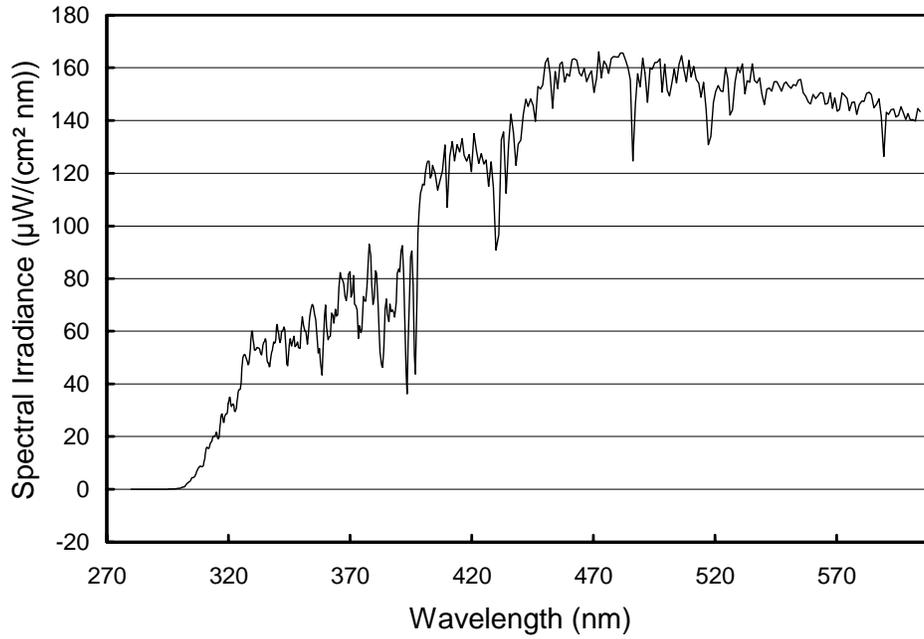
**Figure 3.2.** Irradiance calculated from the PMT currents shown in the previous figure. Data from all three scan items are included.
