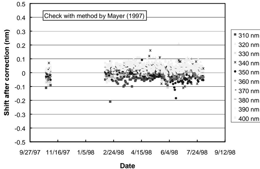
**Figure 3.18.** Check of the wavelength alignment of the Barrow Volume 7 data after applying the Fraunhofer-correlation-based wavelength correction. The check was performed with the method developed by Mayer (1997).
