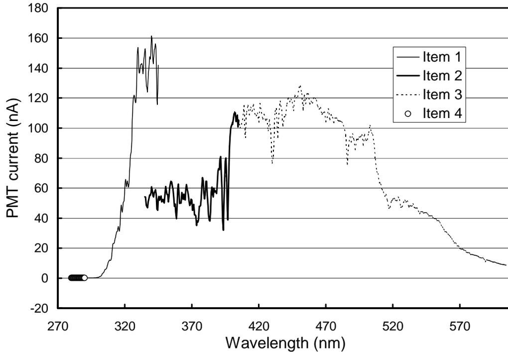
**Figure 3.1.** PMT current before conversion to irradiance. Item 1 covers the spectral range 280-345 nm, Item 2 includes the range 335-405 nm, and Item 3 is from 395 to 605 nm. Item 1 is measured with a higher PMT voltage than Items 2 and 3. Item 4 (280-290 nm) is a measurement of the PMT dark current with the same voltage applied as for Items 2 and 3.
