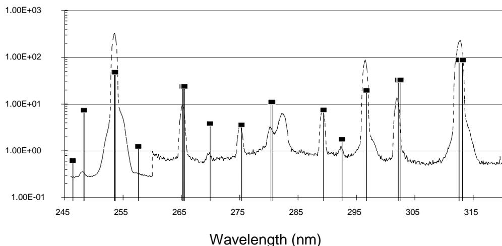
**Figure 3.9.** Example of a Mercury lamp scan with an SUV-100 spectroradiometer (dashed line). Vertical lines represent the positions of the Mercury lines. Lines close together are caused by doublet or triplet emission lines.
