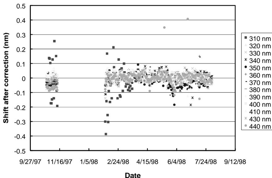
**Figure 3.17.** Check of the wavelength alignment of the Barrow Volume 7 data after applying the Fraunhofer-correlation-based wavelength correction. The check was performed with the method developed by Slaper et al. (1995) using noontime spectra from the 1997/98 season. Similar results have been obtained for all sites.
