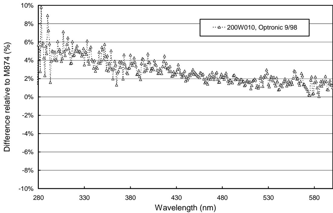
**Figure 3.22.** Comparison of lamps 200W010 and M-874 expressed by the function  $C(\lambda) - 1$ . See text for details. The difference relative to M-874 is positive. This means that solar measurements would increase if 200W010, rather than M-874, were used for calibration.
