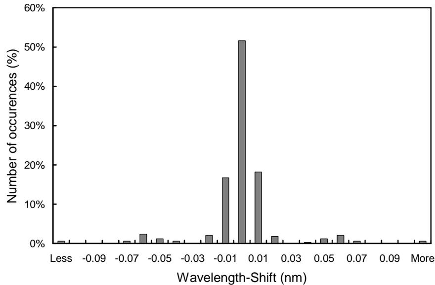
**Figure 3.14.** Differences in the measured position of the 296.728 nm Mercury line between consecutive wavelength scans for Palmer Volume 7. The x-labels give the center wavelength shift for each column. Thus, the 0-nm histogram column covers the range -0.005 to +0.005 nm. “Less” means shifts smaller than -0.105 nm; “more” means shifts larger than 0.105 nm. For 90% of the days, the change in offset is smaller than  $\pm 0.025$  nm.
