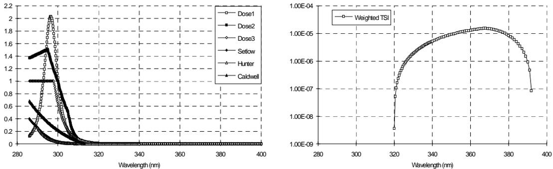
**Figure 3. 23. a-b.** Biological weighting functions (linear axis) and spectral responsivity of the TSI (logarithmic axis).
