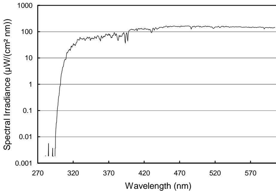
**Figure 3.3.** Spectral irradiance from the previous figure but presented on logarithmic y-axis to demonstrate the steep decline of the solar spectrum in the UV-B.
