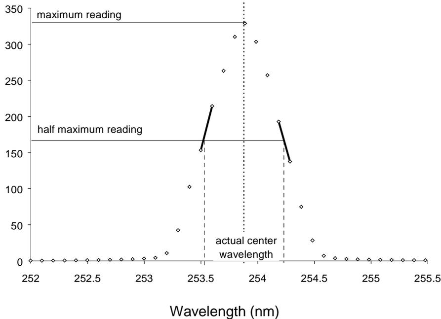
**Figure 3.10.** Details of a single Hg peak along with the illustration of determining the center wavelength using the FWHM method.
