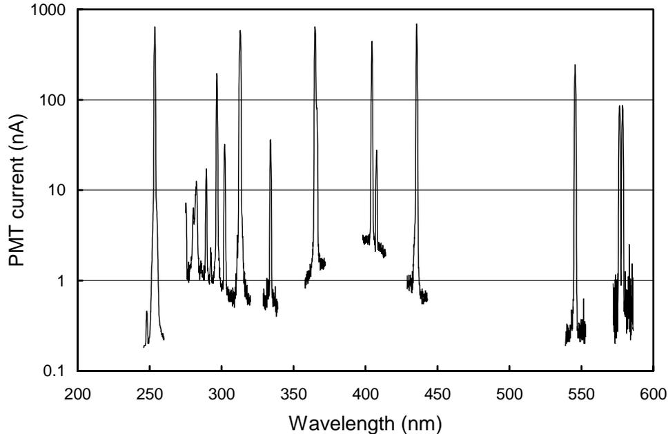
**Figure 3.6.** Typical multi-peak Wavelength scan showing eight segments. The vertical axis indicates PMT current from the Mercury lamp on a logarithmic scale. The dark PMT current has not been subtracted. In a typical wavelength scan, the baseline value may show variation across the spectrum due to fluorescence from the lamp.
