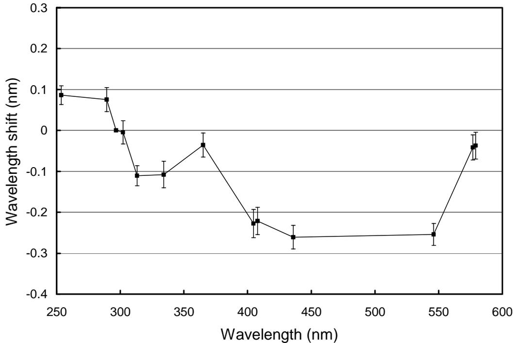
**Figure 3.13.** Typical function expressing monochromator non-linearity. The plot is based on Palmer data from the Volume 7 season. Approximately 347 internal wavelength scans were evaluated. The error bars represent  $\pm 1\sigma$  limits.
