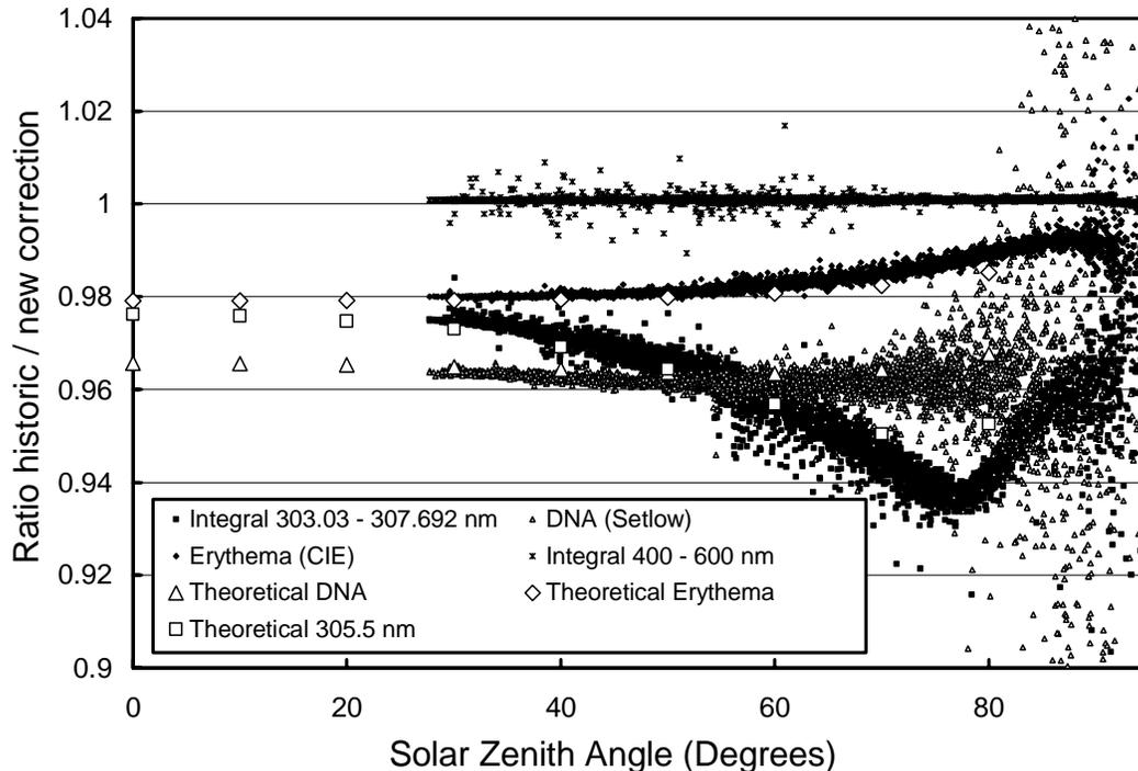
**Figure 3.19.** Effect of the wavelength correction method on spectral integrals. Small symbols show the ratios of data, which were corrected with the historic mercury scan-based method, to data corrected with the new Fraunhofer method. Four different data products are depicted, including the 303.03-307.692 nm and 400-600 nm integrals, as well as erythemally and DNA-weighted irradiance. Large symbols show theoretical results according to Bernhard and Seckmeyer (1999). See text for details.
