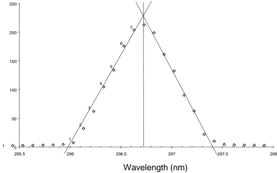
**Figure 3.11.** Implementation of the Tangent method. Diamonds express PMT current of the mercury lamp in the 296-nm peak region. Intersection of the regressions (solid lines) defines center wavelength (dashed line).
