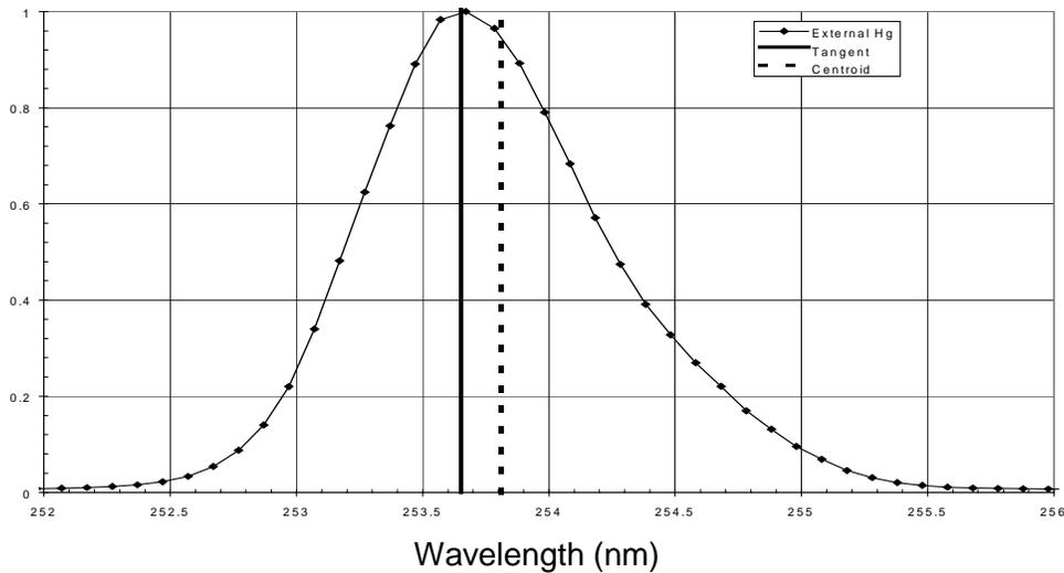
**Figure 3.12.** Differences of the Tangent and Centroid methods. Diamonds express PMT current from the external wavelength scan in the 253 nm peak region; the heavy solid line represents the center wavelength as defined by the tangents method; and the dotted line is the result of the Centroid method. The difference between the two methods (about 0.15 nm) is caused by the well-pronounced right shoulder of the peak.
