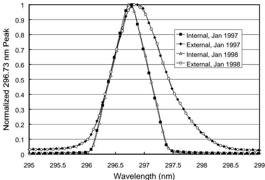
*Figure 3.8. Normalized Mercury peaks from external and internal wavelength scans. Data is from the 1997/98 McMurdo season.*
