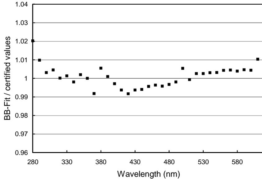
**Figure 3.21.** Ratio of the Black-Body fit values and the certified values of the San Diego site standard 200W010. Both data sets agree to within  $\pm 1\%$ . The graph is based on the same values as shown in the previous figure.
