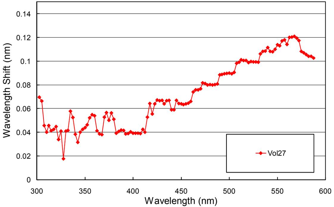
Figure 5.7.5. Monochromator non-linearity correction functions of Volume 27 data.
