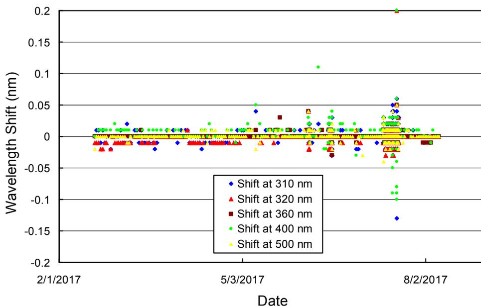
**Figure 5.7.7.** Wavelength accuracy check of “Version 2” Volume 27 data at five wavelengths in the UV and visible by means of Fraunhofer-line correlation. All noontime measurements have been evaluated.
