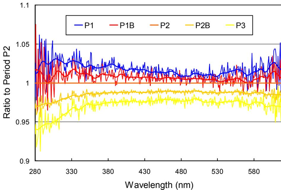
**Figure 5.7.3.** Ratios of irradiance assigned to the internal reference lamp in Periods P1 – P3, referenced to the irradiance of Period P2. Thin lines indicates ratios calculated from the processed lamp spectra. Thick lines are a spline fit to the data. The splined dataset was used for the calibration of solar spectra.
