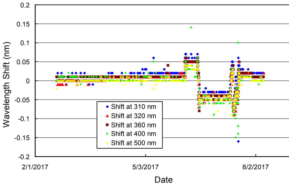
Figure 5.7.6. Wavelength accuracy check of “Version 0” Volume 27 data at five wavelengths in the UV and visible by means of Fraunhofer-line correlation. All noontime measurements have been evaluated.
