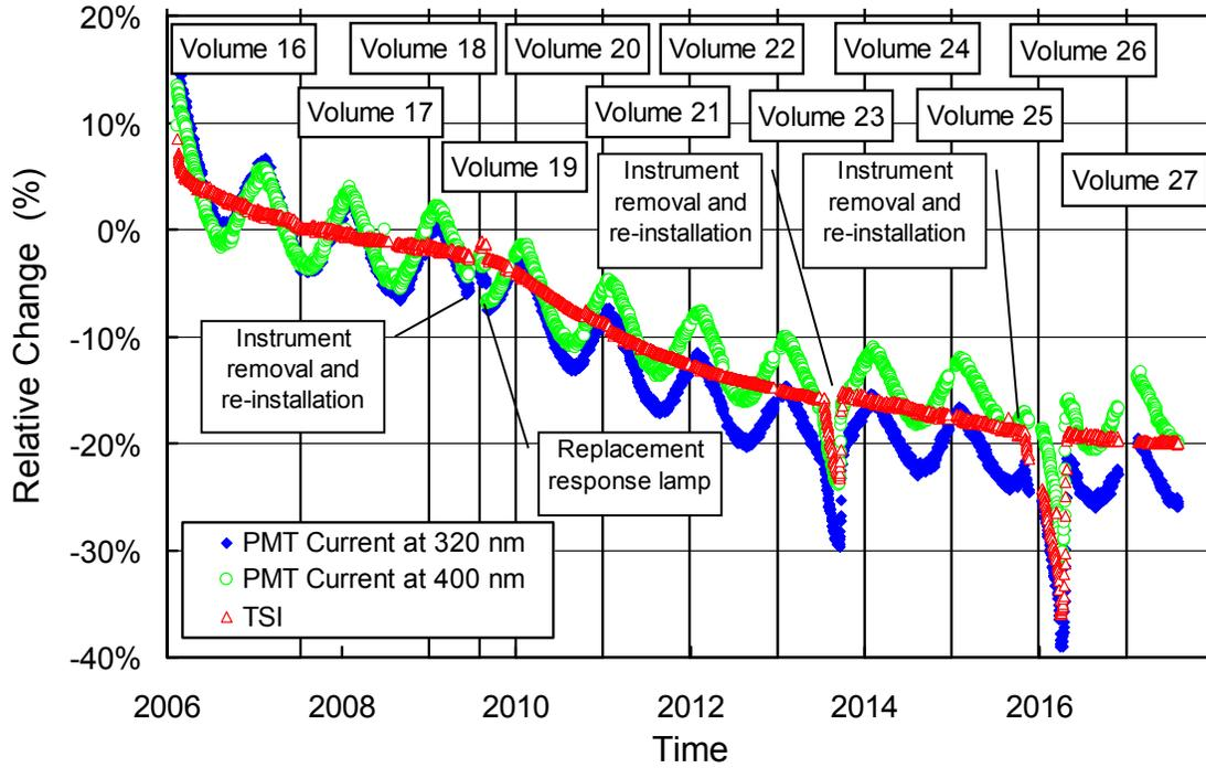
**Figure 5.7.2.** Time-series of TSI signal and PMT currents at 320 and 400 nm during measurements of the internal reference lamp performed at Summit between 2/15/06 and 11/28/16. Data from 9/2/10 (date of response lamp replacement) onward were scaled downward to fit into the existing pattern. Data are normalized to the period 2/14/06 - 6/20/09.
