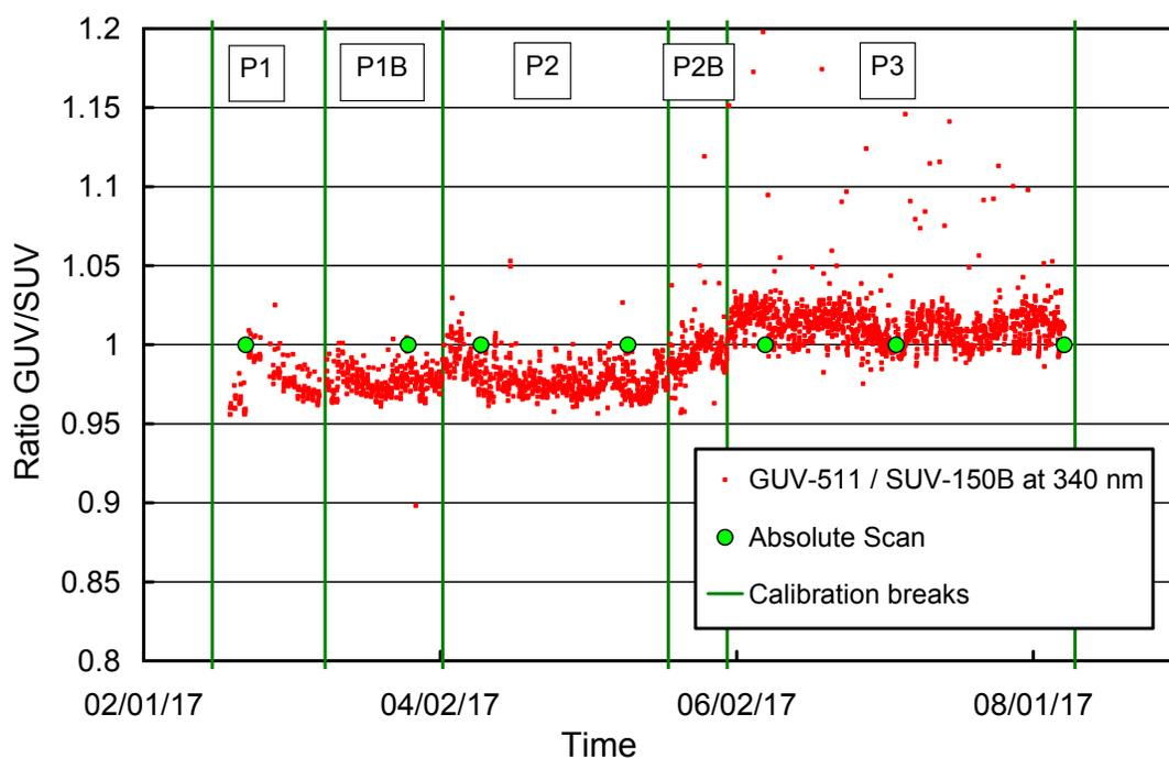
**Figure 5.7.4.** Ratios of GUV-511 and SUV-150B measurements at 340 nm. Breaks in the calibration of SUV data and the times of absolute scans are also indicated. The reason of the apparent 4% step between Periods P2 and P3 is unknown.
