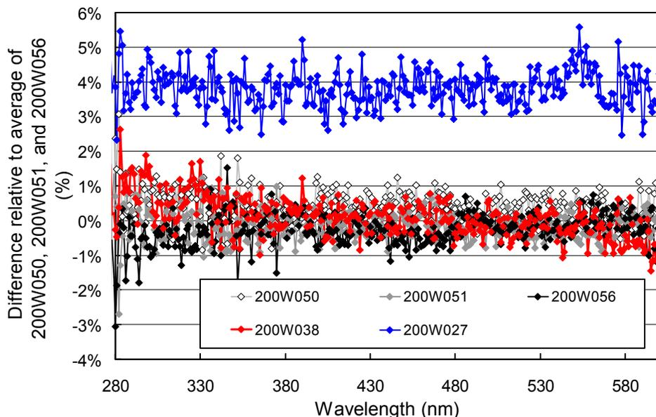
**Figure 5.7.1.** Comparison of San Diego standards 200W050, 200W051, and 200W056 with Summit standards 200W027 and 200W038. Data are referenced to the average of the three San Diego lamps.
