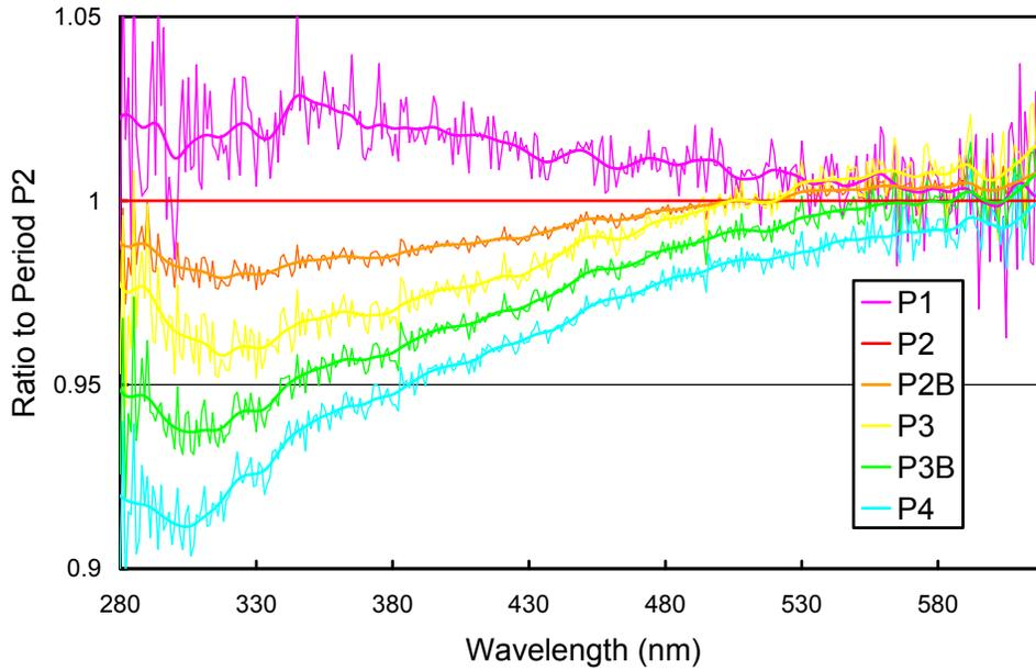
**Figure 5.7.3.** Ratios of irradiance assigned to the internal reference lamp in Periods P1 – P4, referenced to the irradiance of Period P2. At the end of Period P4, the Green House, where the instrument is installed, was moved to a new location. Thick lines indicate ratios of the smoothed irradiance spectra used for the calibration of solar measurements.
