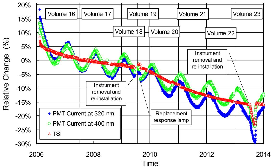
**Figure 5.7.2.** Time-series of TSI signal and PMT currents at 320 nm and 400 nm during measurements of the internal reference lamp performed at Summit between 2/15/06 and 12/31/13. Data from 9/2/10 (date of response lamp replacement) were scaled downward to fit into the existing pattern. Data are normalized to the period 2/14/06 - 6/20/09.
