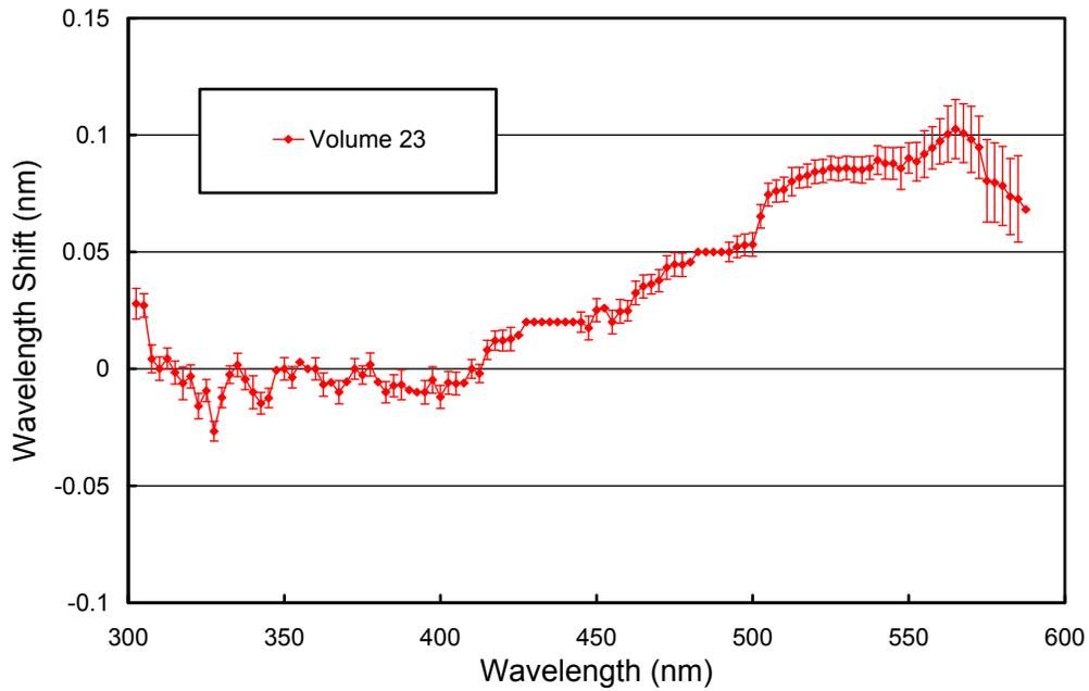
**Figure 5.7.7.** Monochromator non-linearity correction functions of Volume 23 data.
