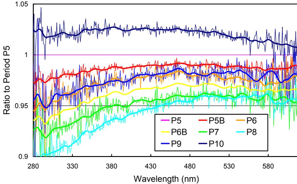
**Figure 5.7.4.** Ratios of irradiance assigned to the internal reference lamp in Periods P5 – P10, referenced to the irradiance of Period P5, which is the first period following the reinstallation of the instrument. Thick lines indicate ratios of the smoothed irradiance spectra used for the calibration of solar measurements.
