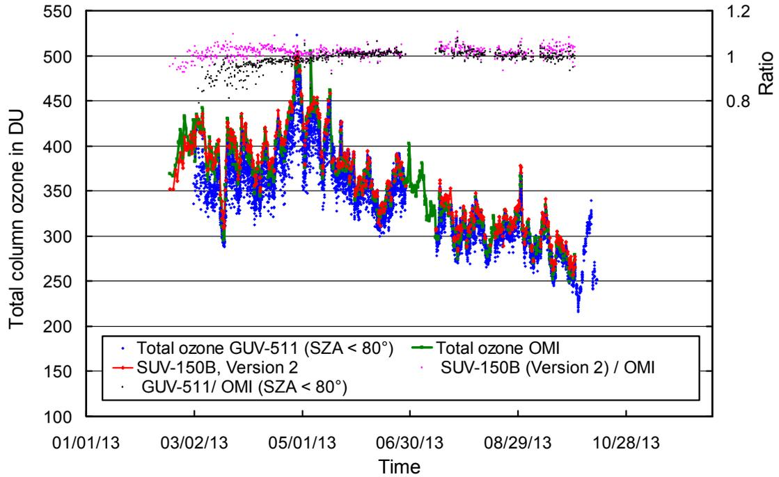
**Figure 5.7.10.** Comparison of total column ozone measurements from GU-511, SUV-150B (Version 2 data), and OMI. GU-511 measurements are plotted in 15 minute intervals. For calculating the ratio of data sets, only measurements concurrent with the OMI overpass were evaluated.
