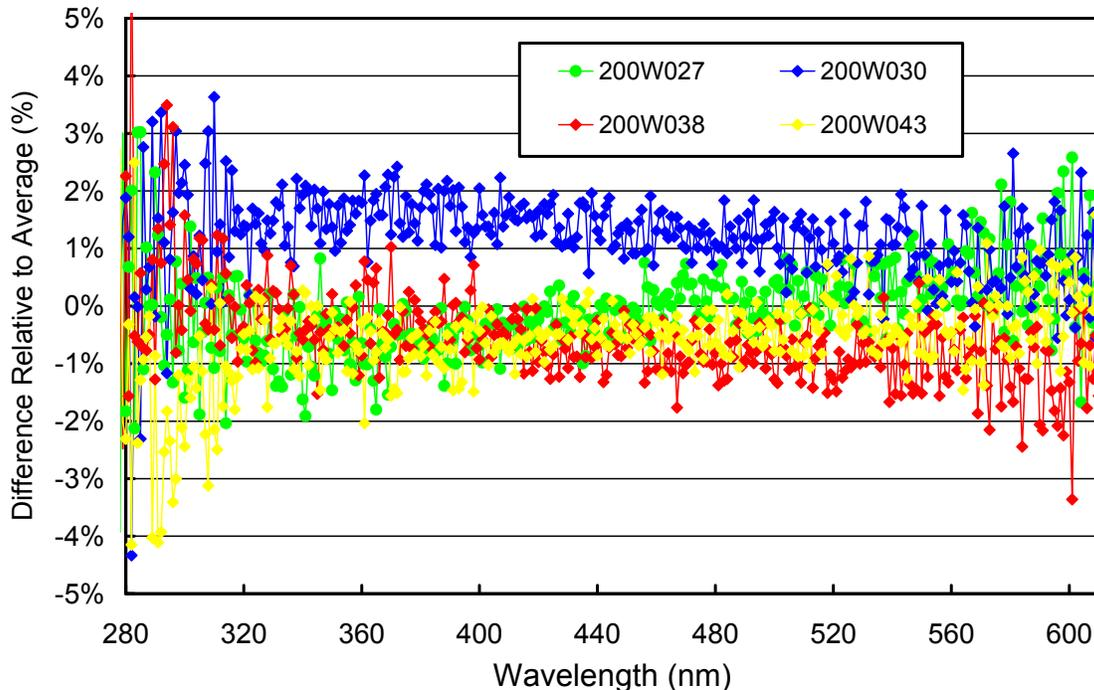
**Figure 5.7.1.** Comparison of lamps 200W027, 200W030, 200W038, and 200W043 on 7/15/2013.
