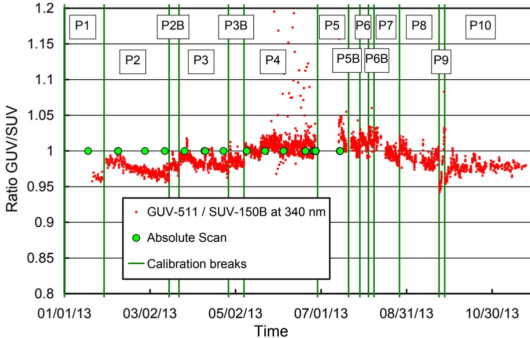
**Figure 5.7.5.** Ratios of GUV-511 and SUV-150B measurements at 340 nm.
