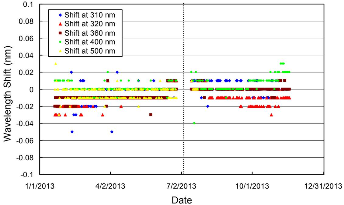
**Figure 5.7.8.** Wavelength accuracy check of “Version 0” Volume 23 data at five wavelengths in the UV and visible by means of Fraunhofer-line correlation. All noontime measurements have been evaluated. The vertical broken line indicates the period when the system was out of operation due to the Greenhouse relocation.
