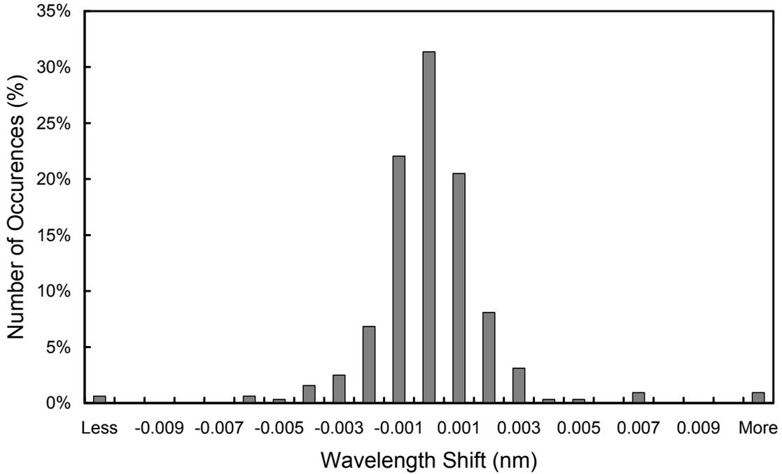
**Figure 5.7.6.** Differences in the measured position of the 296.73 nm mercury line between consecutive wavelength scans for the period 1/1/12 – 12/19/12. The labels of the horizontal axis give the center wavelength shift for each column. The 0-nm histogram column covers the range from -0.0005 to +0.0005 nm. “Less” means shifts smaller than -0.0105 nm; “more” means shifts larger than 0.0105 nm.
