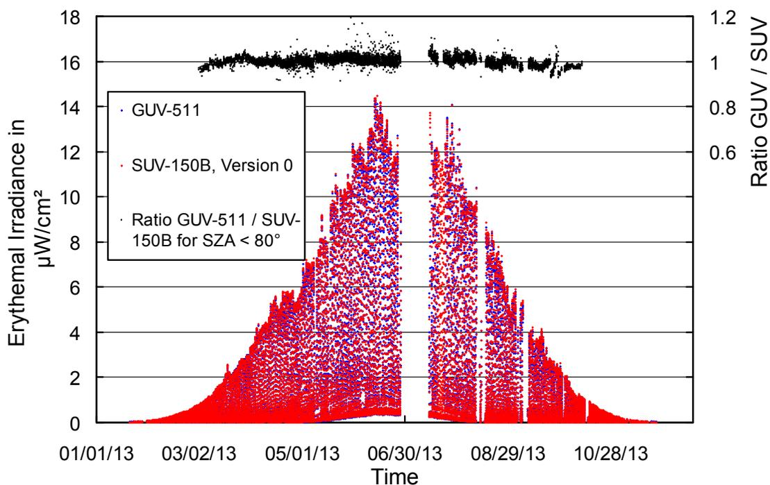
**Figure 5.7.9.** Comparison of erythemal irradiance measured by the SUV-150B spectroradiometer and the GUV-511 radiometer.
