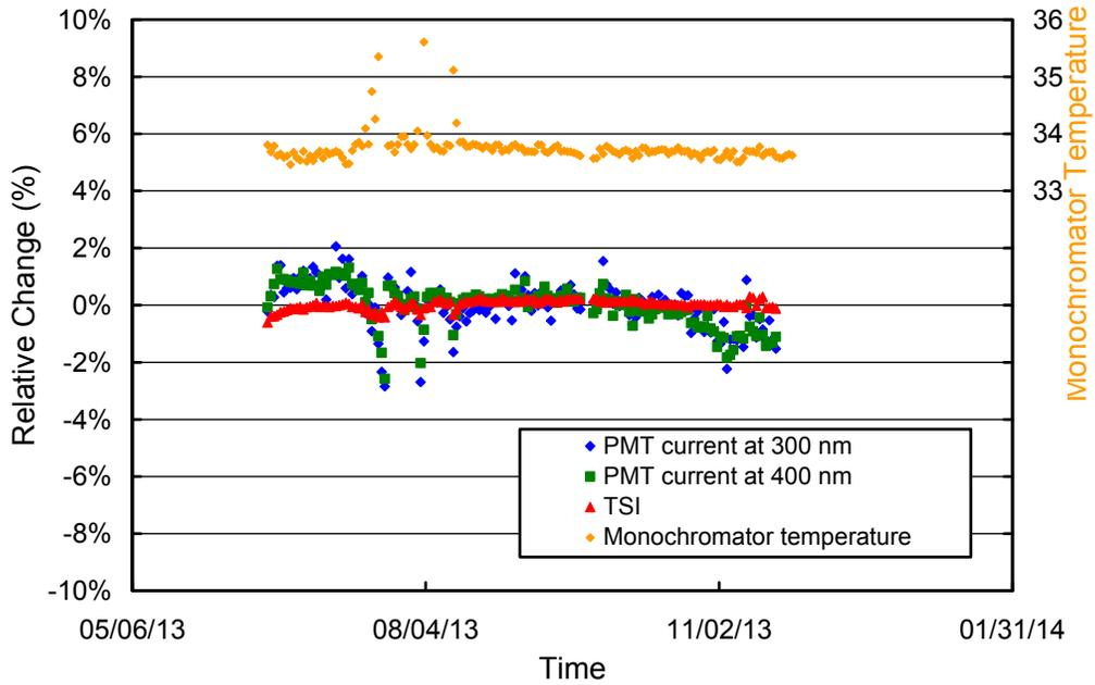
**Figure 5.6.3.** Time-series of PMT current at 300 and 400 nm, and TSI signal measured *after* the site visit. All data were extracted from measurements of the internal irradiance standard and are normalized to their average. Drops in PMT current are apparent at time when the monochromator temperature was elevated.
