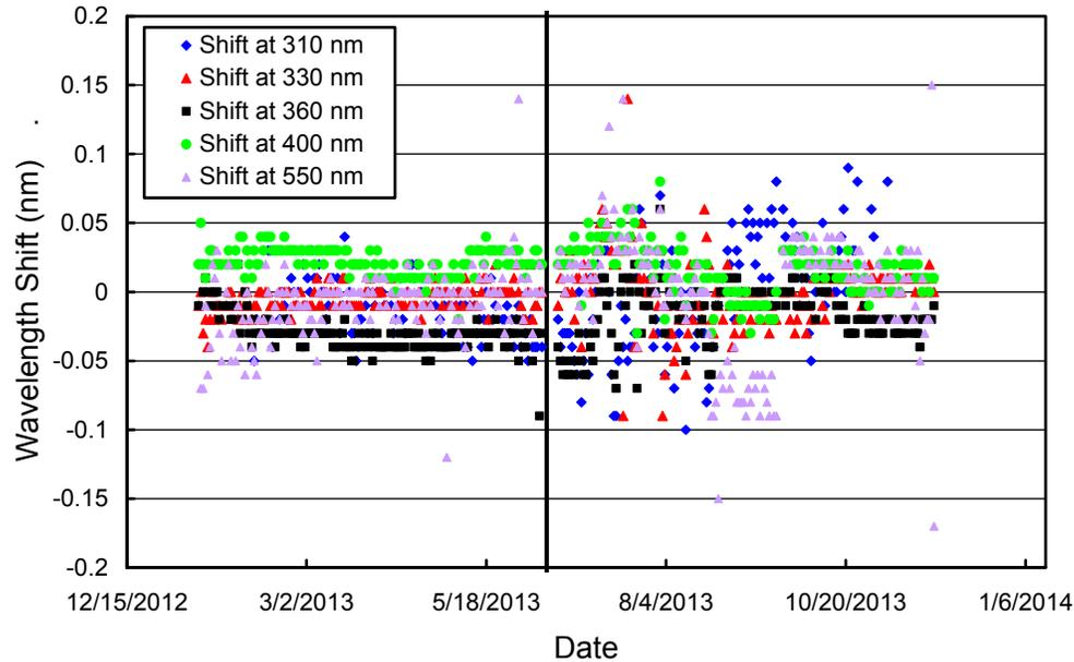
**Figure 5.6.9.** Wavelength accuracy check of final data at four wavelengths in the UV and one in the visible by means of Fraunhofer-line correlation. The noontime measurement has been evaluated for each day of the reporting period when the Sun was above the horizon. The vertical black line marks the time of the site visit.
