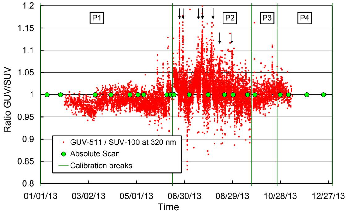
**Figure 5.6.6.** Ratio of GUV-511 measurements of the 320-nm channel to SUV-100 measurements. The latter were weighted with the spectral response function of the 320-nm GUV-511 channel. Times of absolute scans and calibration breaks are also indicated. Arrows indicate the periods listed in Table 1 when SUV measurements were low.
