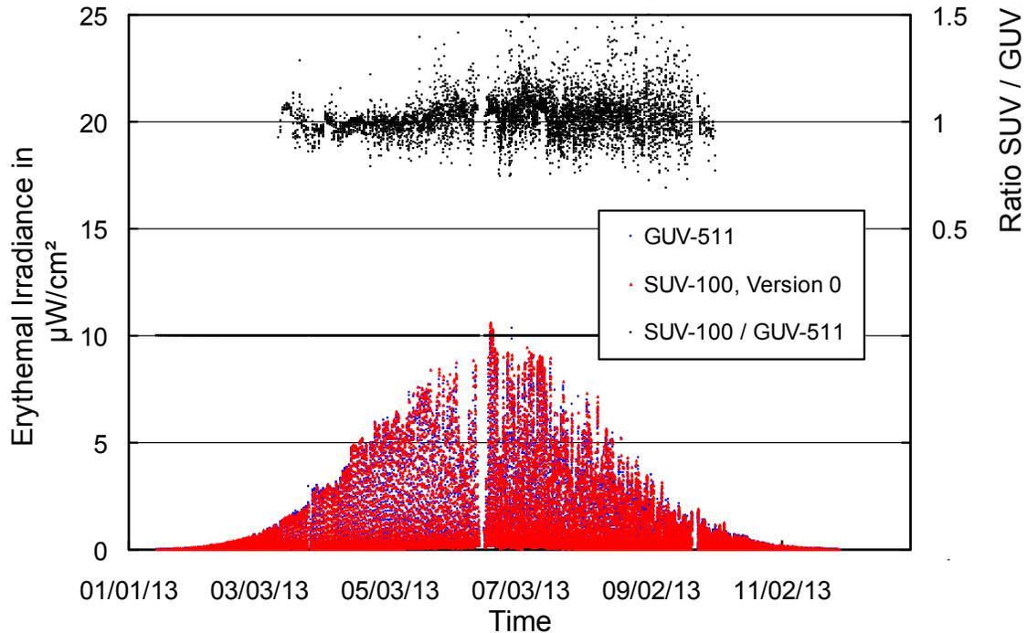
**Figure 5.6.10.** Comparison of erythemal irradiance measured by the SUV-100 spectroradiometer and the GUV-511 radiometer. Data are based on “Version 0” (cosine-error uncorrected) data.
