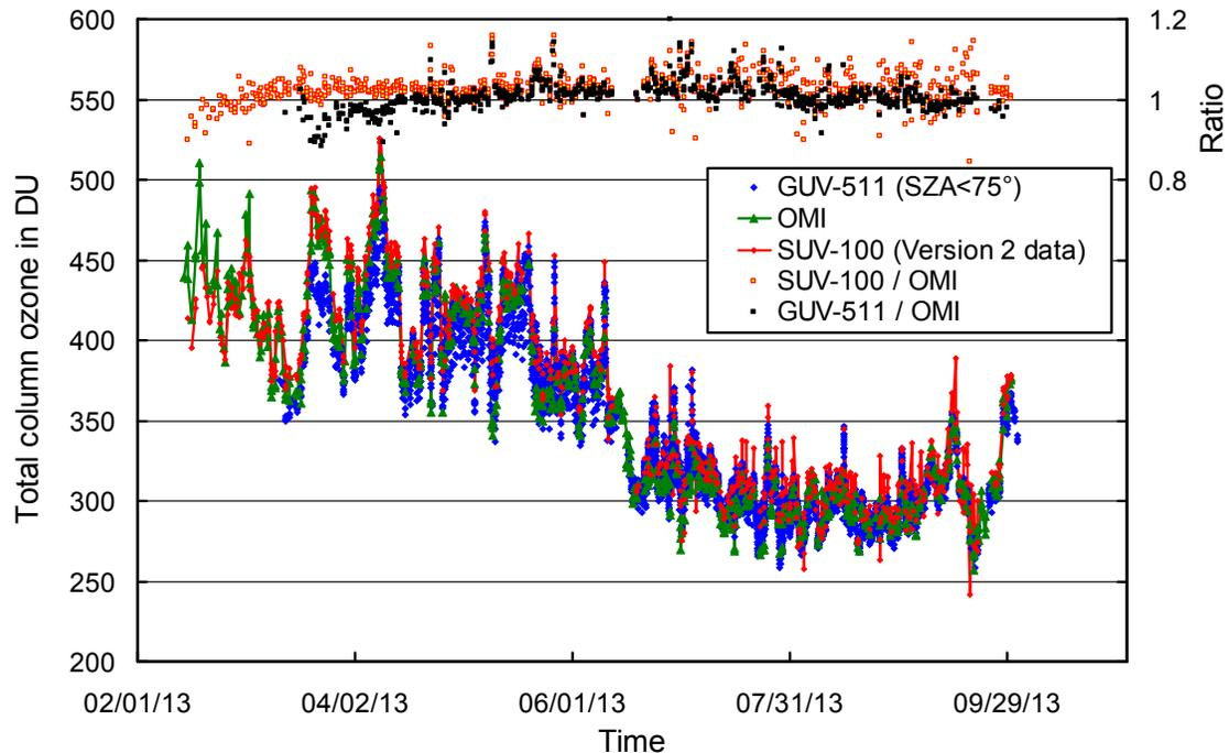
**Figure 5.6.11.** Comparison of total column ozone measurements from GUV-511, OMI, and SUV-100. GUV-511 measurements are plotted in 30 minute intervals. For calculating the ratios of SUV-100/OMI and GUV-511/OMI, only measurements concurrent with the OMI overpass were evaluated.
