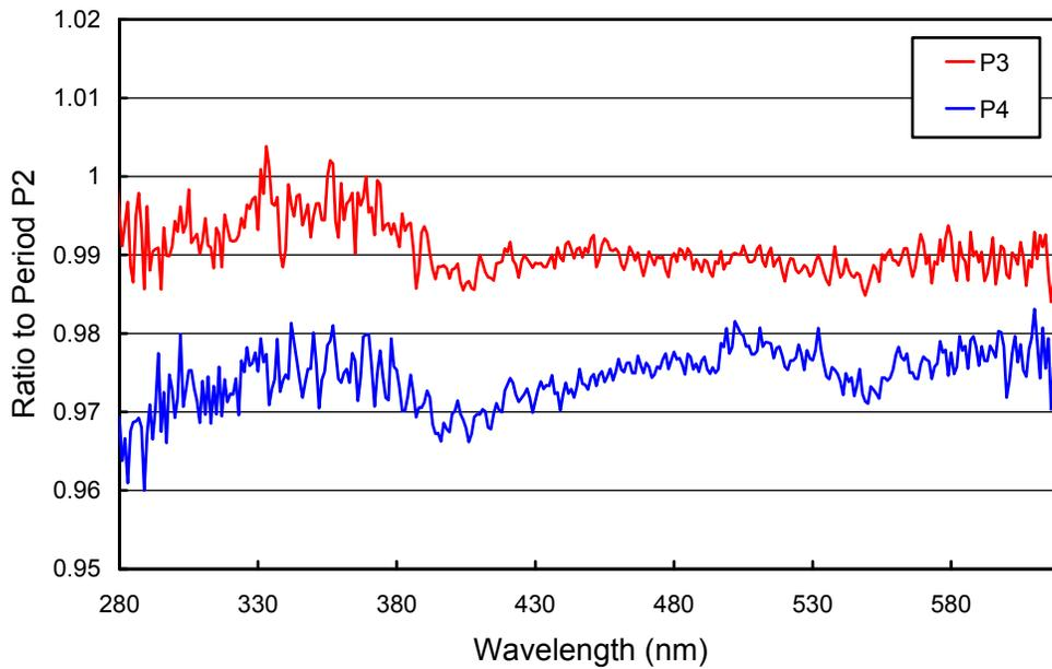
**Figure 5.6.4.** Ratios of spectral irradiance assigned to the internal reference lamp during the Periods P3 and P4, relative to Period P2.
