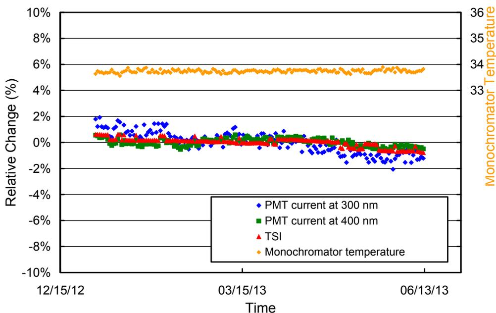
**Figure 5.6.2.** Time-series of PMT current at 300 and 400 nm, and TSI signal measured *before* the site visit. All data were extracted from measurements of the internal irradiance standard and are normalized to their average.
