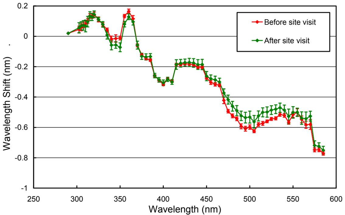
**Figure 5.6.8.** Monochromator non-linearity correction functions for Barrow Volume 23. Error bars indicate the standard deviation of the data contributing to this plot.
