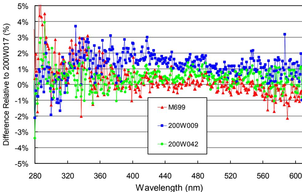
**Figure 5.6.1.** Comparison of on-site lamps M-699, 200W009, and 200W042 with traveling standard 200W017 on 6/12/13.
