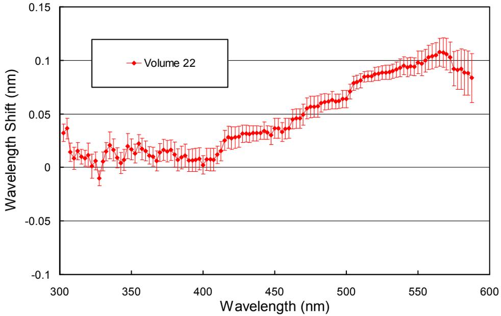
**Figure 5.7.9.** Monochromator non-linearity correction functions of Volume 22 data.
