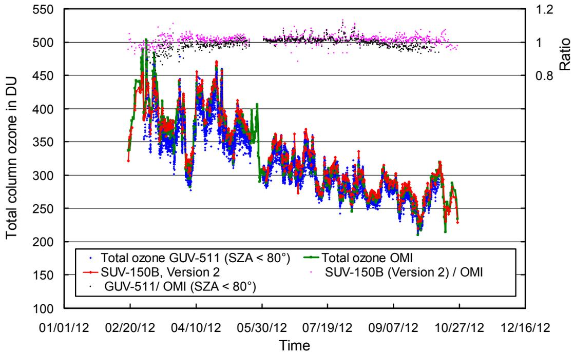
**Figure 5.7.12.** Comparison of total column ozone measurements from GUV-511, SUV-150B (Version 2 data), and OMI. GUV-511 measurements are plotted in 15 minute intervals. For calculating the ratio of data sets, only measurements concurrent with the OMI overpass were evaluated.
