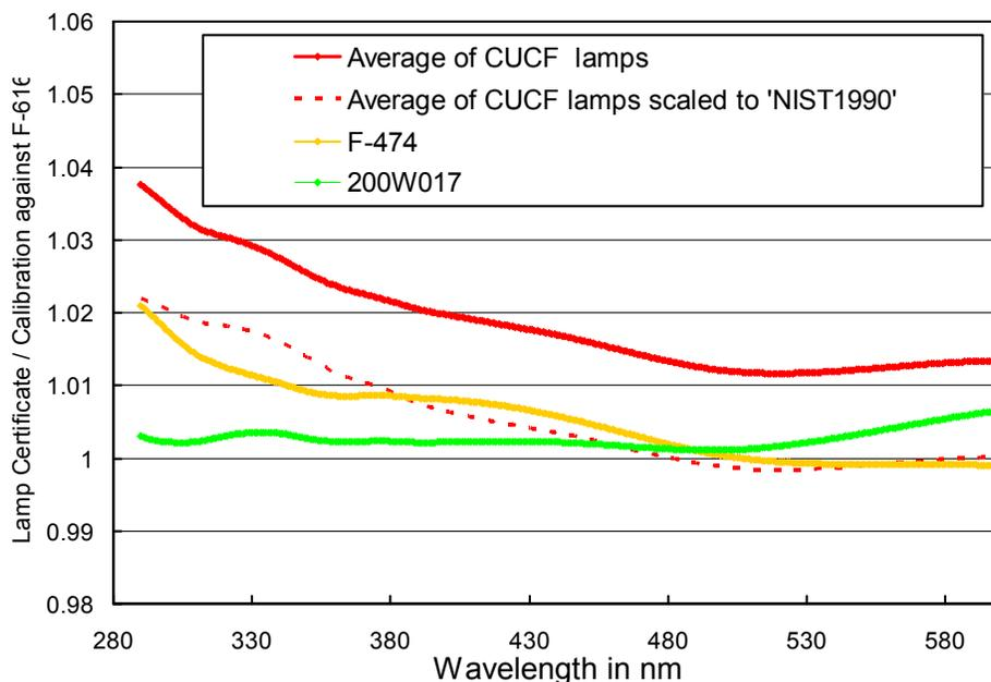
**Figure 5.7.1.** Irradiance scale of CUCF lamps, NIST lamp F-474, and traveling standard 200W017 relative to irradiance scale of NIST standard F-616. The ratio indicated by the dotted red line was constructed by scaling the scale of the CUCF lamps to the NIST1990 scale and comparing the result with the scale represented by NIST standard F-616.
