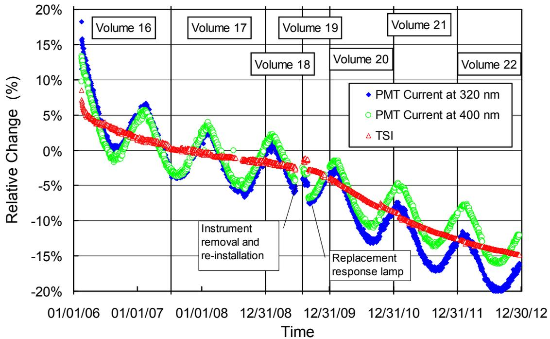
**Figure 5.7.3.** Time-series of TSI signal and PMT currents at 320 nm and 400 nm during measurements of the internal reference lamp performed at Summit between 2/15/06 and 12/31/12. Data from 9/2/10 (date of response lamp replacement) were scaled to downward to fit into the existing pattern.
