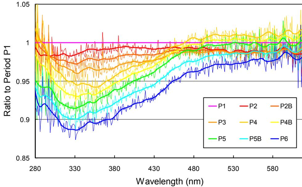
**Figure 5.7.4.** Ratios of irradiance assigned to the internal reference lamp in Periods P2 – P6, referenced to the irradiance of Period P1. At the end of Period P6, the Green House where the instrument is installed was releveled. Thick lines indicate ratios of the smoothed irradiance spectra used for the calibration of solar measurements.
