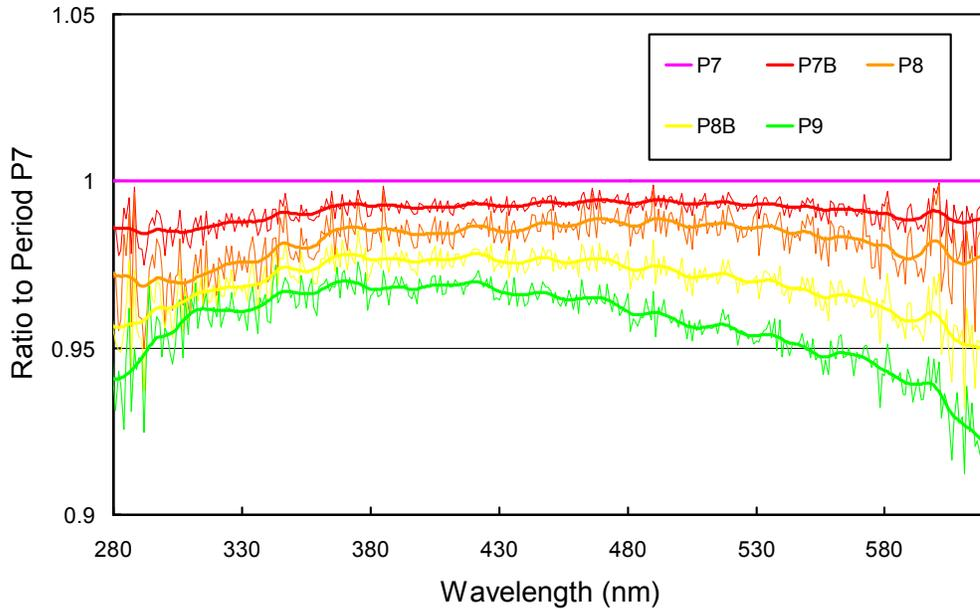
**Figure 5.7.5.** Ratios of irradiance assigned to the internal reference lamp in Periods P7 – P9, referenced to the irradiance of Period P7, which is the first period following the leveling of the Green House. Thick lines indicate ratios of the smoothed irradiance spectra used for the calibration of solar measurements.
