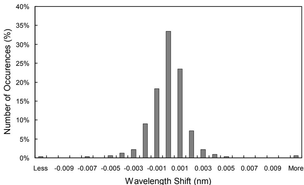
**Figure 5.7.8.** Differences in the measured position of the 296.73 nm mercury line between consecutive wavelength scans for the period 1/1/12 – 12/19/12. The labels of the horizontal axis give the center wavelength shift for each column. The 0-nm histogram column covers the range from  $-0.0005$  to  $+0.0005$  nm. "Less" means shifts smaller than  $-0.0105$  nm; "more" means shifts larger than  $0.0105$  nm.
