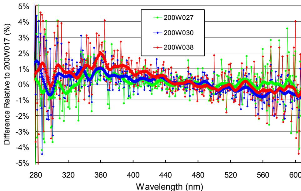
**Figure 5.7.2.** Comparison of lamps 200W027, 200W030, and 200W038 with 200W017 on 3-4 November 2011. Heavy solid lines indicate smoothed data.
