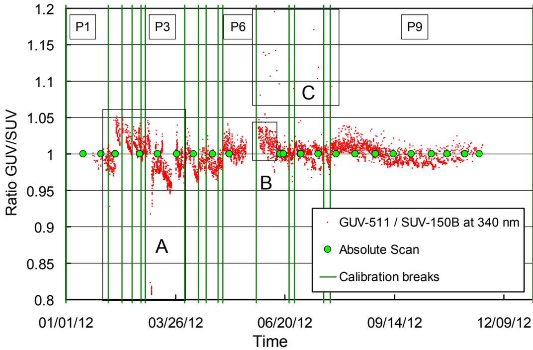
**Figure 5.7.6.** Ratios of GUV-511 and SUV-150B measurements at 340 nm. Period A is shown in greater detail in Figure 5.7.7.
