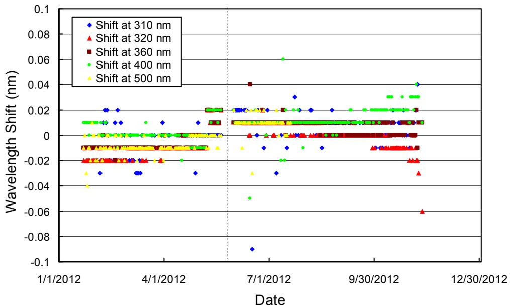
**Figure 5.7.10.** Wavelength accuracy check of final Volume 22 data at five wavelengths in the UV and visible by means of Fraunhofer-line correlation. All noontime measurement have been evaluated. The vertical broken line indicates the day when the Green House was releaved.
