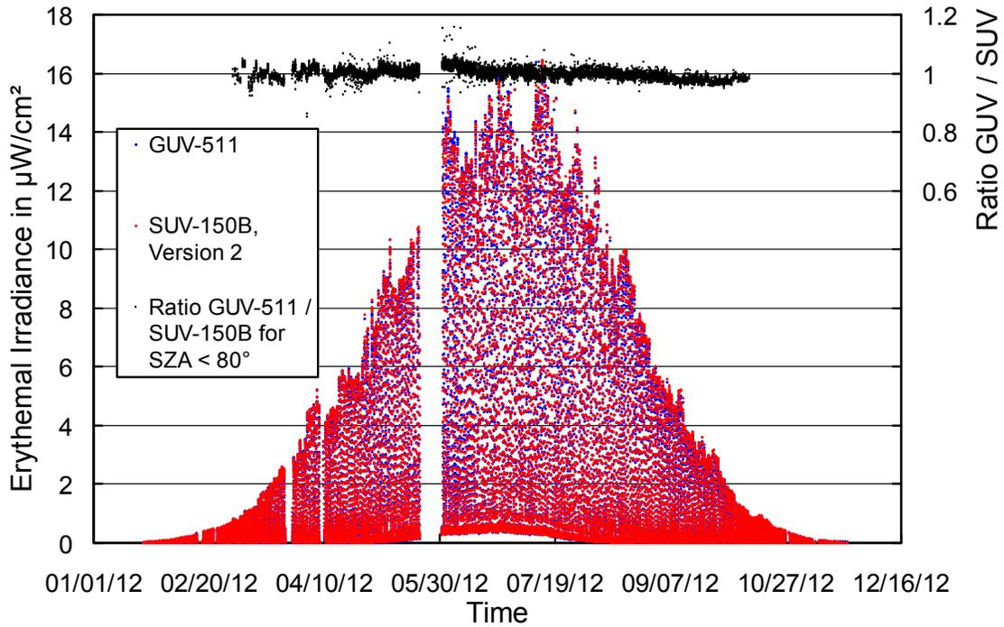
**Figure 5.7.11.** Comparison of erythemal irradiance measured by the SUV-150B spectroradiometer and the GUV-511 radiometer. SUV-150B measurements are based on “Version 2” (cosine-error corrected) data.
