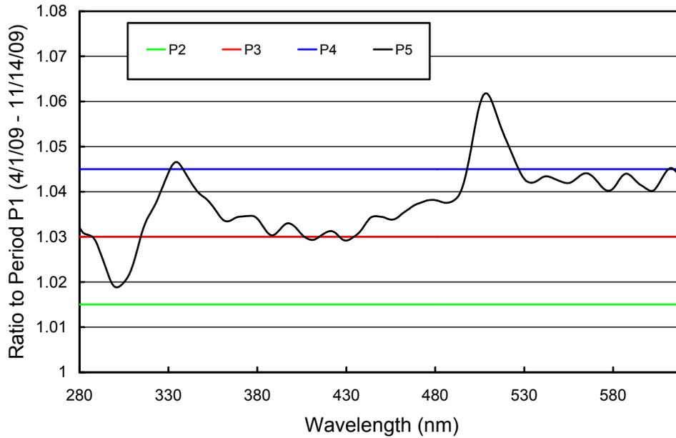
**Figure 5.1.4** Ratios of irradiance assigned to the internal reference lamp during periods P2 – P5, relative to Period P1.
