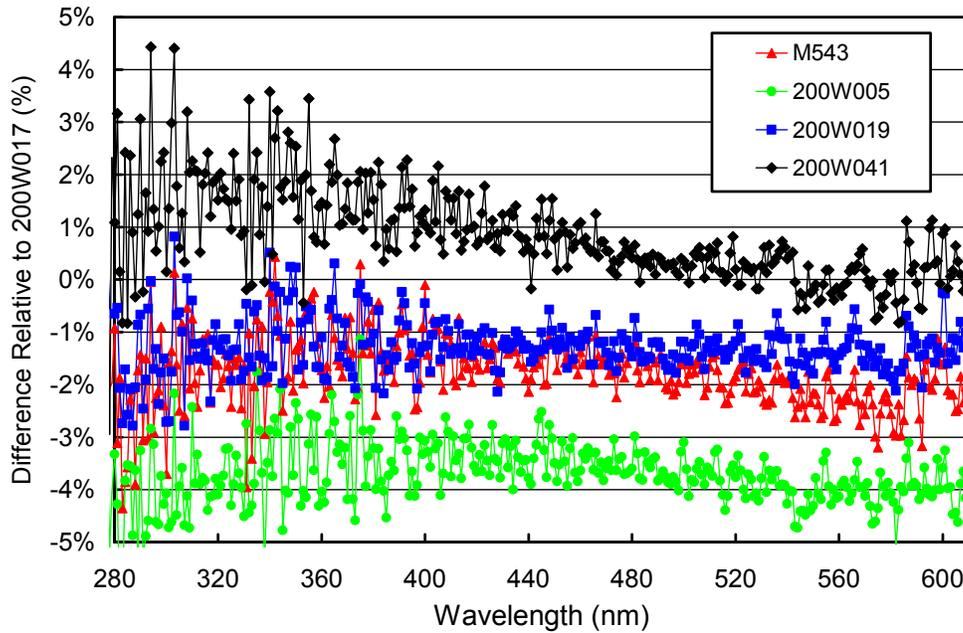
**Figure 5.1.1.** Comparison of McMurdo lamps M-543, 200W005, 200W019 and 200W041 with the BSI traveling standard 200W017 on 2/11/09.
