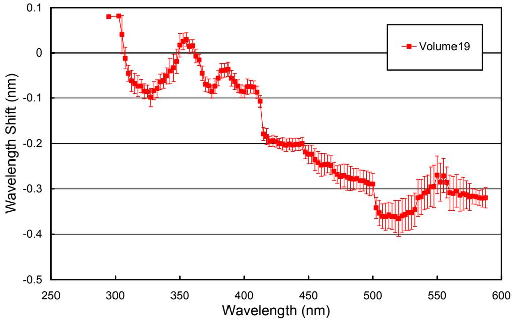
**Figure 5.1.5.** Monochromator non-linearity correction function. Error bars indicate the  $1\sigma$ -variation.
