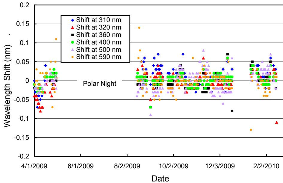
**Figure 5.1.6.** Check of the wavelength accuracy of final data at four wavelengths by means of Fraunhofer-line correlation. The noontime measurement has been evaluated for each day of the season. No correlation data is available during Polar Night. No data are available between 12/19/10 and 1/12/10.
