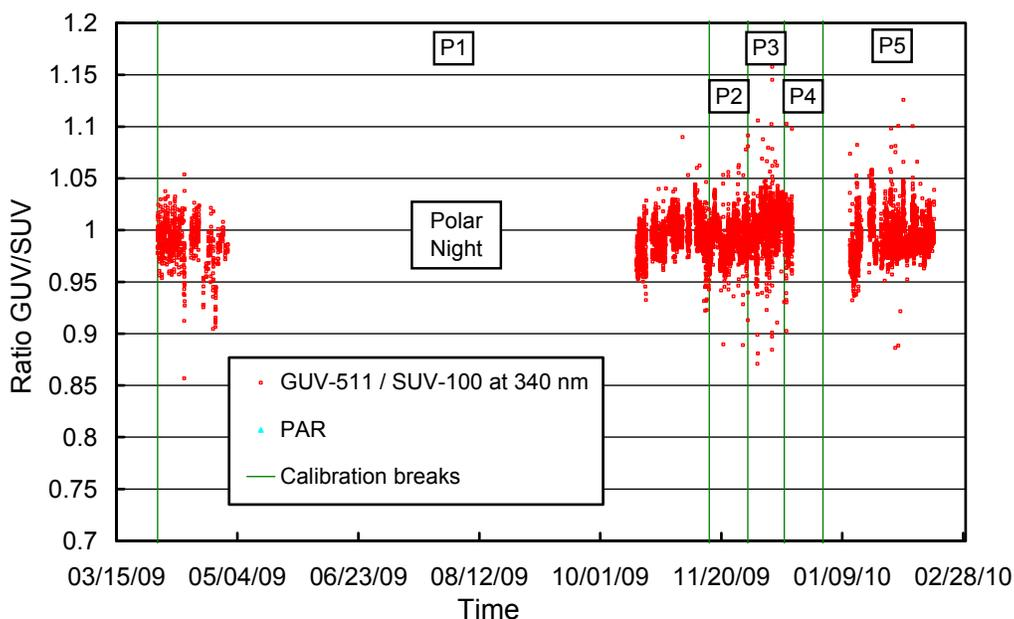
**Figure 5.1.3.** Ratio of GUV-511 measurements of its 340 nm channel with final SUV-100 measurements that were weighted with the spectral response function of this channel.
