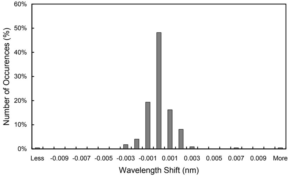
**Figure 5.7.6.** Differences in the measured position of the 296.73 nm mercury line between consecutive wavelength scans for the period 8/15/04 – 5/12/05. The labels of the horizontal axis give the center wavelength shift for each column. The 0-nm histogram column covers the range from -0.0005 to +0.0005 nm. “Less” means shifts smaller than -0.0105 nm; “more” means shifts larger than 0.0105 nm.
