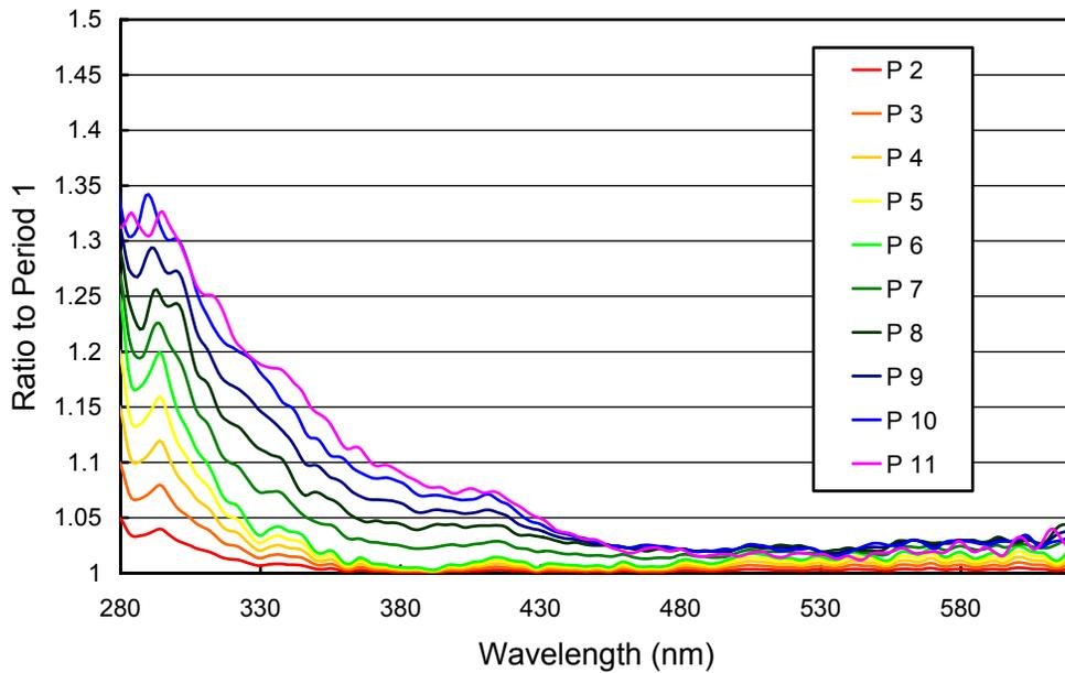
**Figure 5.7.4.** Ratios of irradiance assigned to the internal reference lamp in Periods P 2 – P 11, referenced to the irradiance of Period P 1. All calibration functions were smoothed with an approximating spline.
