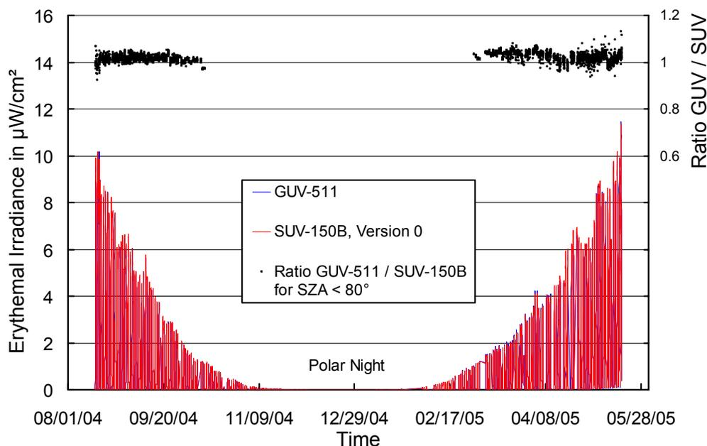
**Figure 5.7.9.** Comparison of erythemal irradiance measured by the SUV-150B spectroradiometer and the GUV-511 radiometer. SUV-150B measurements are based on “Version 0” (cosine-error uncorrected) data.
