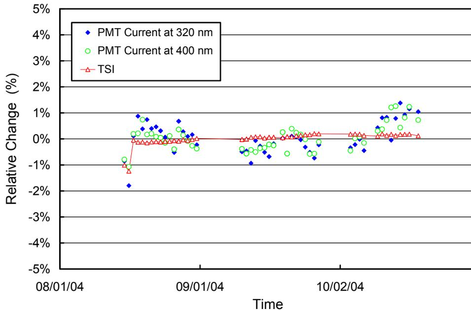
**Figure 5.7.2.** Time-series of TSI signal and PMT currents at 320 and 400 nm during measurements of the internal reference lamp performed at Summit between 8/15/04 and 10/19/04. On 10/20/04, the response lamp stopped functioning due to an intermitted circuit.
