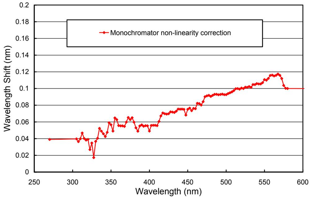
**Figure 5.7.7.** Monochromator non-linearity correction functions for the Volume 14 period at Summit.
