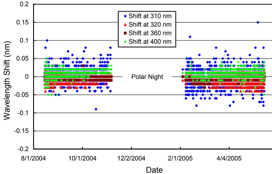
**Figure 5.7.8.** Wavelength accuracy check of final data at four wavelengths in the UV by means of Fraunhofer-line correlation. All measurement at solar zenith angles larger than 89° have been evaluated.
