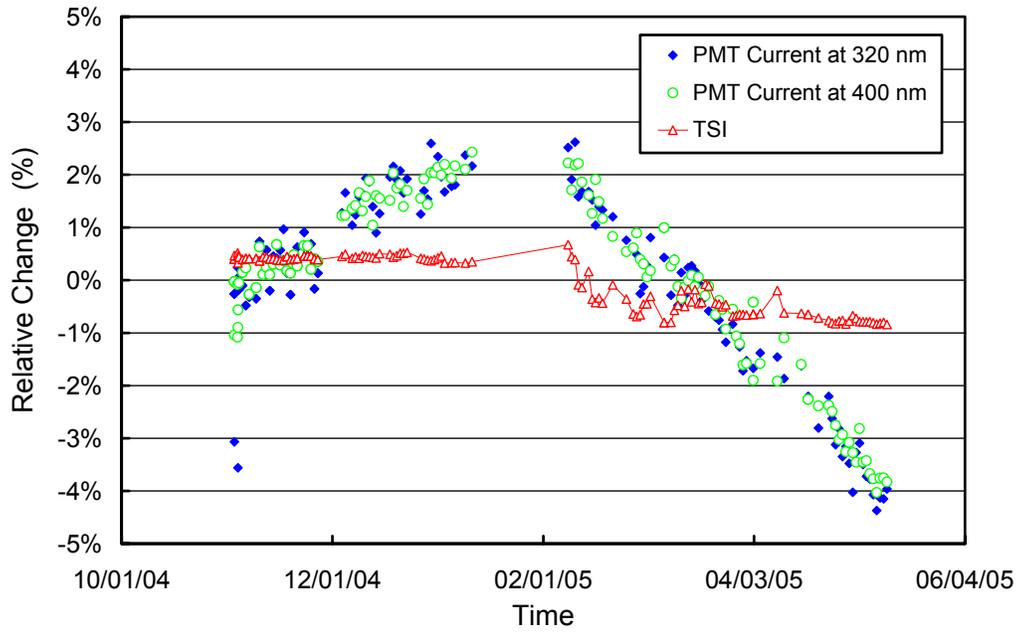
**Figure 5.7.3.** Time-series of TSI signal and PMT currents at 320 and 400 nm during measurements of the internal reference lamp performed at Summit between 11/2/04 and 5/12/05. This period covers the interval when the 2<sup>nd</sup> response lamp was installed.
