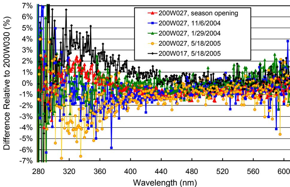
**Figure 5.7.1.** Comparison of lamps 200W027 and 200W017 with lamp 200W030 at Summit.
