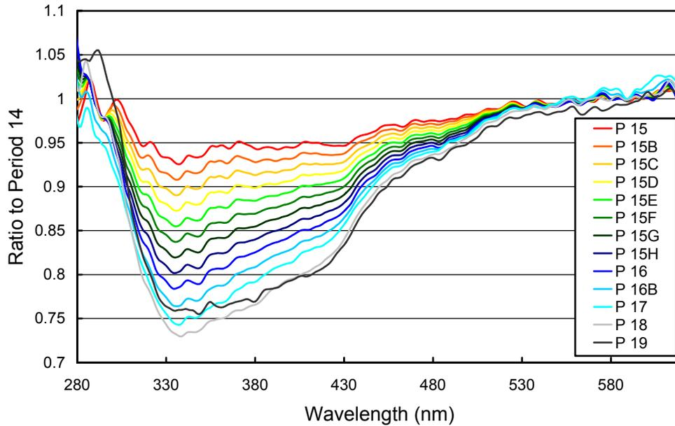
**Figure 5.7.5** Ratios of irradiance assigned to the internal reference lamp in Periods P 15 - P 19, referenced to the irradiance of Period P 14. All calibration functions were smoothed with an approximating spline.
