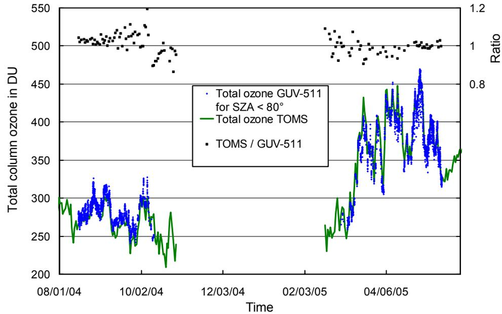
**Figure 5.7.10.** Comparison of total column ozone measurements from GUV-511 and NASA/TOMS Earth Probe satellite. GUV-511 measurements are plotted in 15 minute intervals. For calculating the ratio of both data sets, only GUV-511 measurements concurrent with the TOMS overpass data were evaluated.
