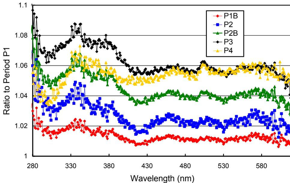
**Figure 5.6.5.** Ratios of spectral irradiance values assigned to the internal reference lamp during the Periods P1B–P4 to Period P1.
