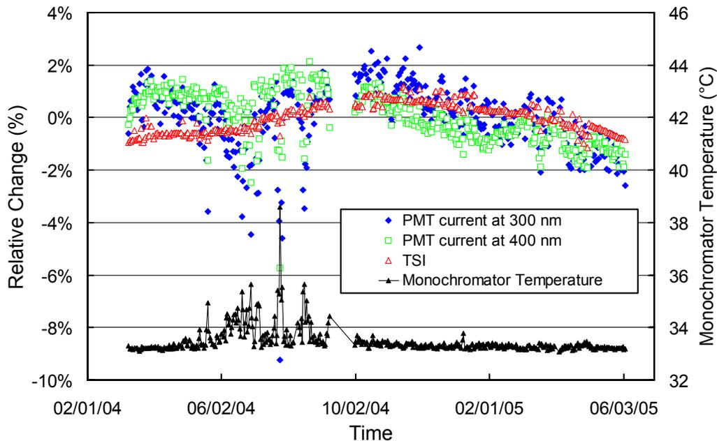
**Figure 5.6.3.** Left axis: Time-series of PMT current at 300 and 400 nm, and TSI signal extracted from measurements of the internal irradiance standard at Barrow between 3/9/04 – 6/4/05. All data sets are normalized to the average. Right axis: Monochromator temperature.
