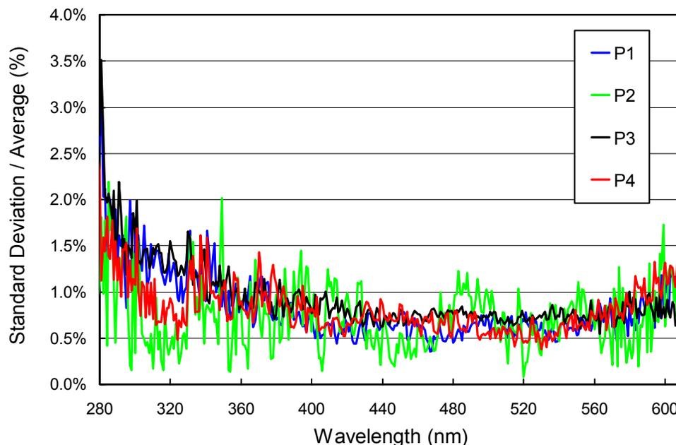
**Figure 5.6.6.** Ratio of standard deviation and average spectra calculated from absolute calibration scans.
