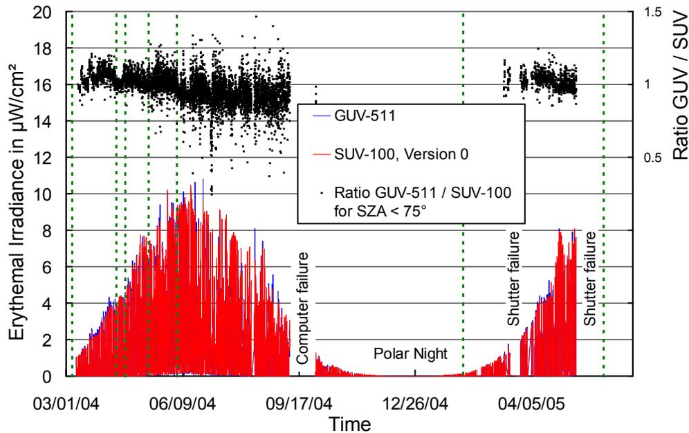
**Figure 5.6.11.** Comparison of erythemal irradiance measured by the SUV-100 spectroradiometer and the GUV-511 radiometer. All data is based on “Version 0” (cosine-error uncorrected) data.
