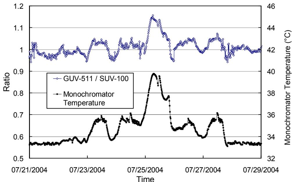
**Figure 5.6.4.** Left axis: Ratio of GUV-511 measurements of the 340-nm channel to SUV-100 measurements weighted with the spectral response function of the 340-nm GUV-511 channel. Right axis: Monochromator temperature.
