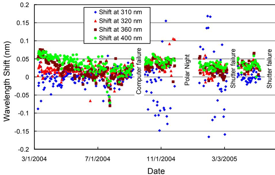
**Figure 5.6.9.** Wavelength accuracy check of final data at four wavelengths in the UV by means of Fraunhofer-line correlation. The noontime measurement has been evaluated for each day of the reporting period when the Sun was above the horizon. No data are available for periods affected by computer and shutter failures, and during Polar Night.
