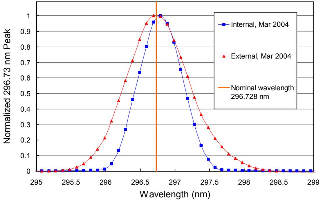
**Figure 5.6.10.** The 296.73 mercury line as registered by the PMT from external and internal sources at the start of the reporting period. The wavelength scale is the same as applied for solar measurements.
