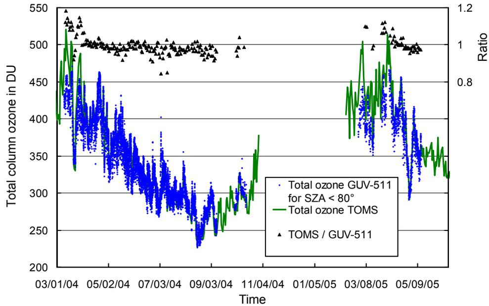
**Figure 5.6.12.** Comparison of total column ozone measurements from GUV-511 and NASA/TOMS Earth Probe satellite. GUV-511 measurements are plotted in 15 minute intervals. For calculating the ratio of both data sets, only GUV-511 measurements concurrent with the TOMS overpass data were evaluated.
