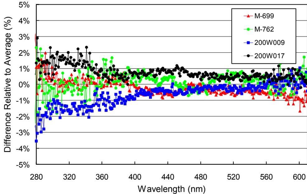
**Figure 5.6.1.** Comparison of lamps 200W009, M-762, M-699, and 200W017 at the beginning of the Volume 14 period.
