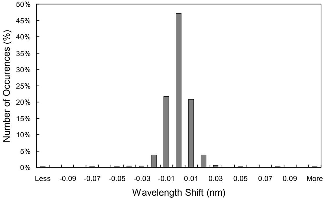
**Figure 5.6.7.** Differences in the measured position of the 296.73 nm mercury line between consecutive wavelength scans. The x-labels give the center wavelength shift for each column. Thus the 0-nm histogram column covers the range -0.005 to +0.005 nm. “Less” means shifts smaller than -0.105 nm; “more” means shifts larger than 0.105 nm.
