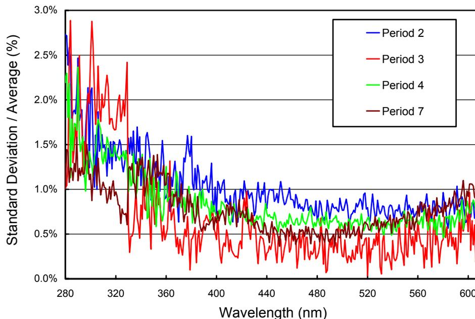
**Figure 5.5.5.** Ratio of standard deviation and average calculated from the absolute calibration scans used to establish the calibration of the San Diego spectroradiometer for the 2002-2003 season. Only period with at least three absolute scans are shown.
