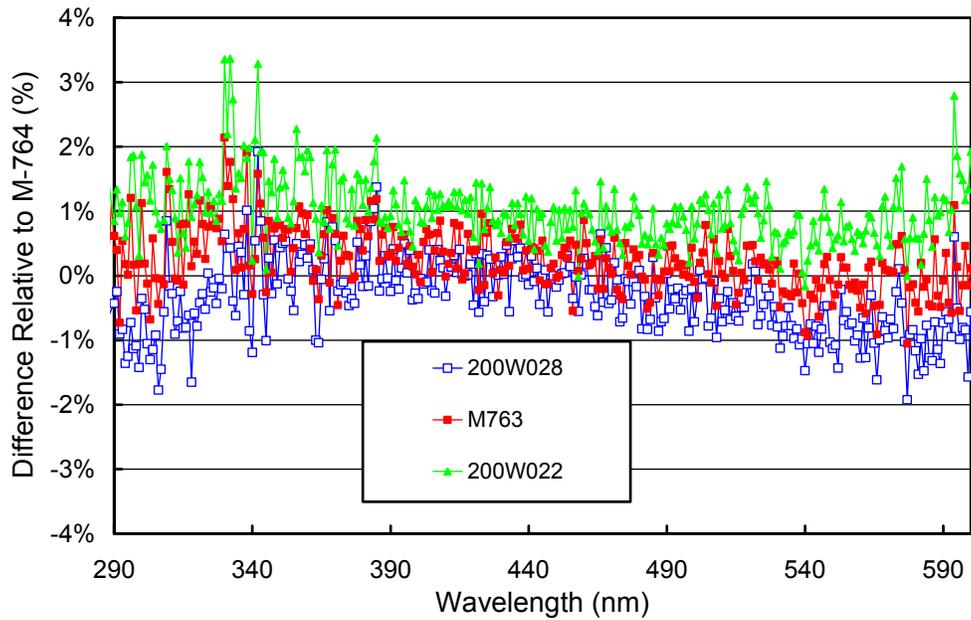
**Figure 5.5.2.** Comparison of 200W028, M-763, and 200W022 with M-764 in May 2002
