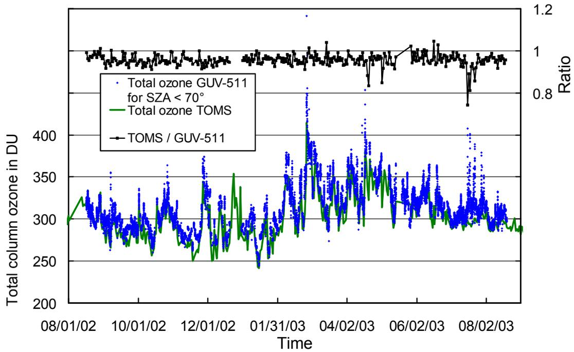
**Figure 5.5.11.** Comparison of total column ozone measurements from GUV-511 and NASA/TOMS Earth Probe satellite. GUV-511 measurements are plotted in 15 minute intervals. For calculating the ratio of both data sets only GUV-511 measurements coincident with the TOMS overpass were evaluated.
