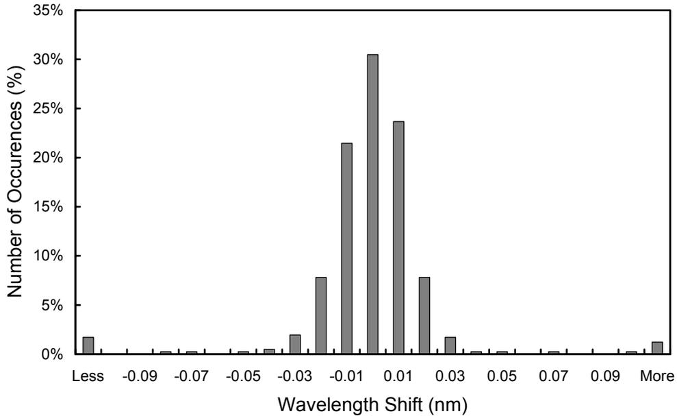
**Figure 5.5.6.** Differences in the measured position of the 296.73 nm mercury line between consecutive wavelength scans. The x-labels give the center wavelength shift for each column. The 0-nm histogram column covers the range -0.005 to +0.005 nm. “Less” means shifts smaller than -0.105 nm; “more” means shifts larger than 0.105 nm.
