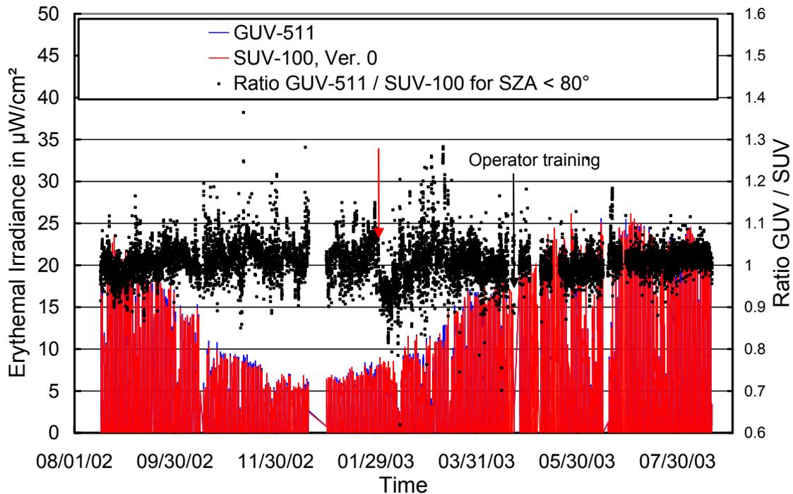
**Figure 5.5.10.** Comparison of erythemal irradiance measured by the SUV-100 spectroradiometer and the GUV-511 radiometer. All data is based on “Version 0” (cosine-error uncorrected) data. See text for explanation of the step indicated by the red arrow.
