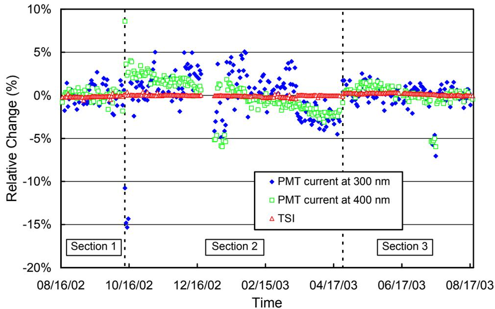
**Figure 5.5.3.** Time-series of PMT current at 300 and 400 nm, and TSI signal during measurements of the internal irradiance reference lamp during the San Diego 2002–2003 season. The data is normalized to the average value of each of the three sections indicated in the graph.
