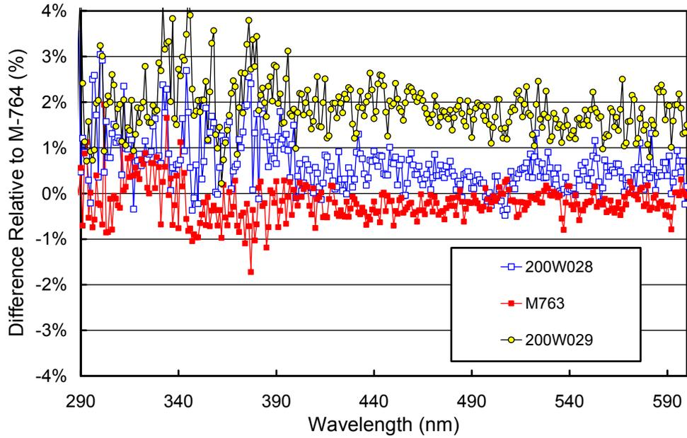
**Figure 5.5.1.** Comparison of 200W028, 200W029, and M-763 with the traveling standard M-764 in September 2002.
