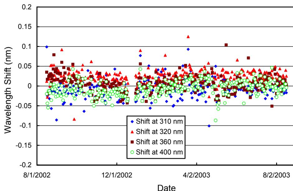
**Figure 5.5.8.** Check of the wavelength accuracy of the final data at four wavelengths by means of Fraunhofer correlation. The noontime measurements have been evaluated for each day of the season.
