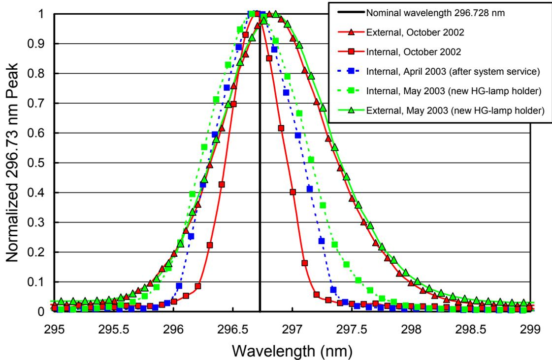
Figure 5.5.9. The 296.73 mercury line as registered by the PMT from external and internal sources.
