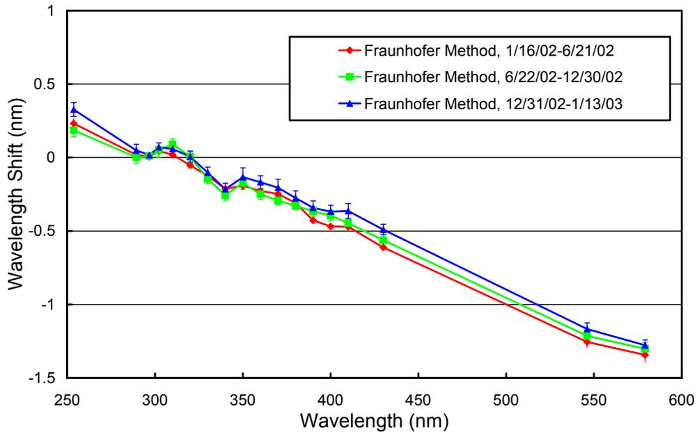
**Figure 5.3.7.** Monochromator non-linearity functions for the South Pole 2002/03 season. The error bars show the 1 $\sigma$  standard deviation of the wavelength shifts.
