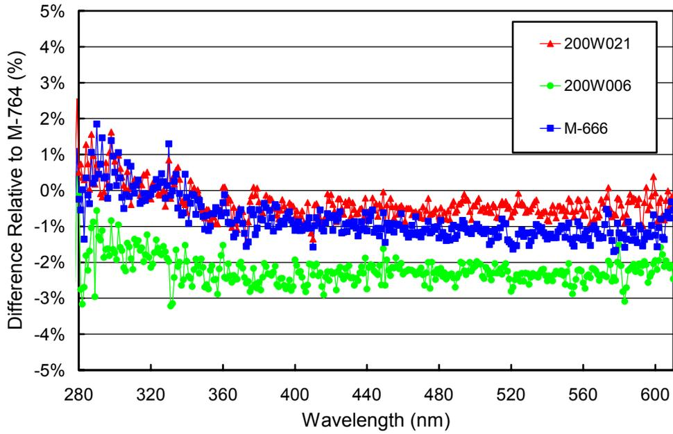
**Figure 5.3.1.** Comparison of South Pole lamps 200W006, 200W021, and M-666 with the BSI traveling standard M-764 at the start of the season on 1/18/02.
