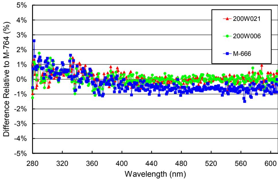
**Figure 5.3.2.** Comparison of South Pole lamps 200W006, 200W021, M-666 with the BSI traveling standard M-764 at the end of the season on 1/11/03 and 1/12/03.
