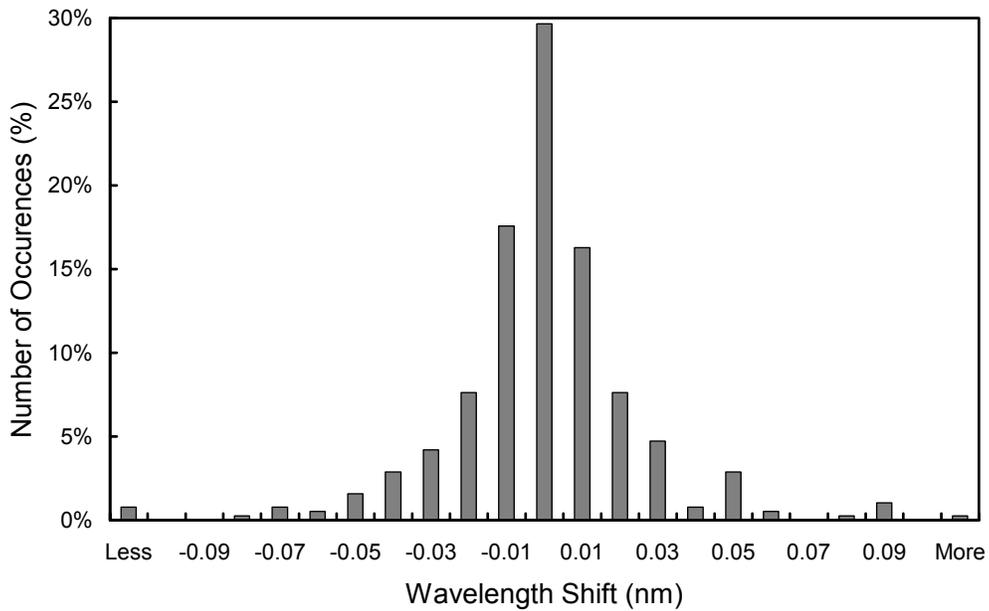
**Figure 5.3.6.** Differences in the measured position of the 296.73 nm mercury line between consecutive wavelength scans. The x-labels give the center wavelength shift for each column. The 0-nm histogram column covers the range -0.005 to +0.005 nm. “Less” means shifts smaller than -0.105 nm; “more” means shifts larger than 0.105 nm.
