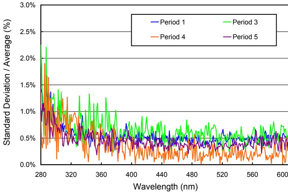
**Figure 5.3.5.** Ratio of standard deviation and average calculated from the absolute calibration scans measured during the South Pole 2002/03 season.
