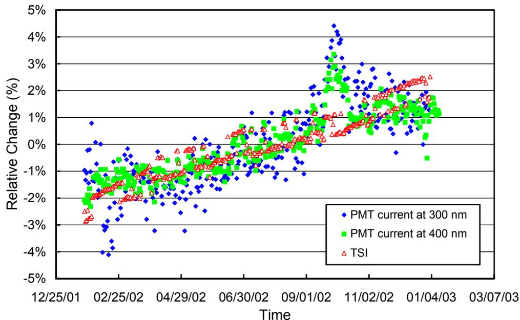
**Figure 5.3.3.** Time-series of PMT current at 300 and 400 nm, and TSI signal during measurements of the internal irradiance standard performed during the South Pole 2002/03 season. The data are normalized to the average of the whole period.
