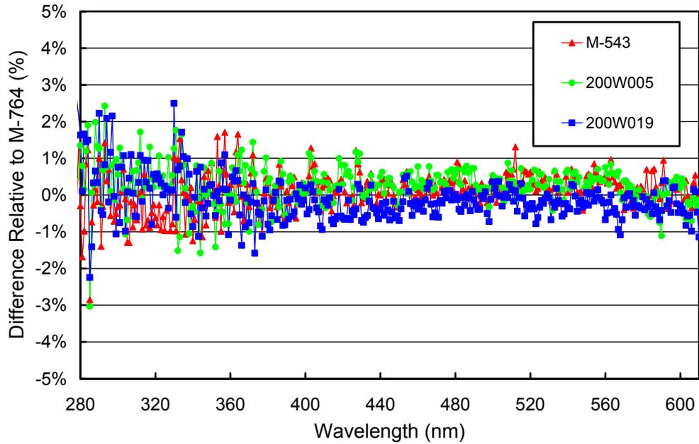
**Figure 5.1.2.** Comparison of McMurdo lamps M-543, 200W005, and 200W019 with the BSI traveling standard M-764 at the beginning of the season (1/25/02-1/26/02).
