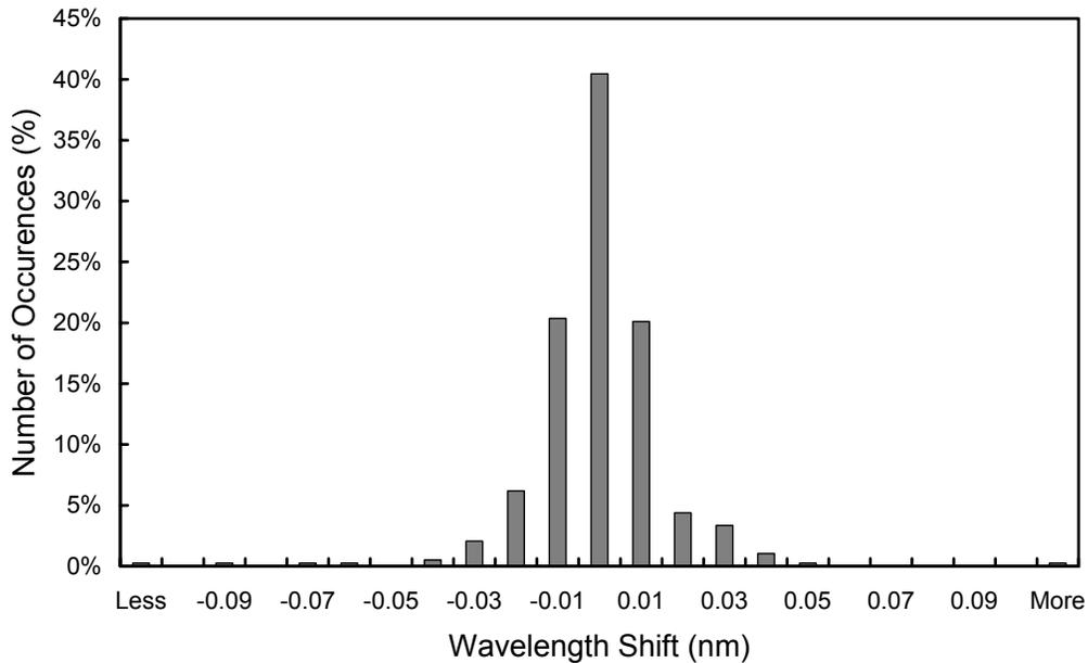
**Figure 5.1.7.** Differences in the measured position of the 296.73 nm mercury line between consecutive wavelength scans. The x-labels give the center wavelength shift for each column. The 0-nm histogram column covers the range  $-0.005$  to  $+0.005$  nm. “Less” means shifts smaller than  $-0.105$  nm; “more” means shifts larger than  $0.105$  nm.
