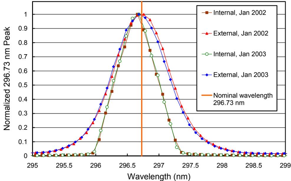
**Figure 5.1.10** The 296.73 mercury line as registered by the PMT from external and internal sources. The wavelength scale is the same as applied for solar measurements, i.e., it is based on a combination of internal scans and the Fraunhofer-correlation method. It is assumed that the wavelength registration of the monochromator did not shift between internal and external scans, which were close in time.
