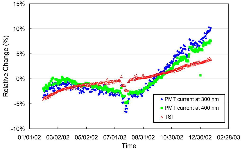
**Figure 5.1.4.** Time-series of PMT current at 300 and 400 nm, and TSI signal during measurements of the internal irradiance reference lamp during the McMurdo 2002/03 season. The data is normalized to the average value of the whole season.
