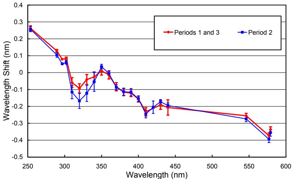
**Figure 5.1.8.** Monochromator non-linearity correction functions for McMurdo 2002/03 data. The functions were calculated with the Fraunhofer-correlation method. Period 1 covers the period 1/24/02-12/26/02, Period 2 is 12/27/02-1/2/03 and Period 3 is 1/3/03-1/25/03.
