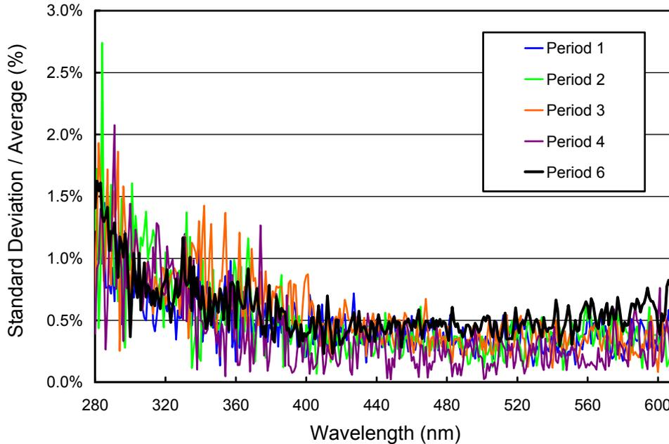
**Figure 5.1.6.** Ratio of standard deviation and average calculated from the absolute calibration scans.
