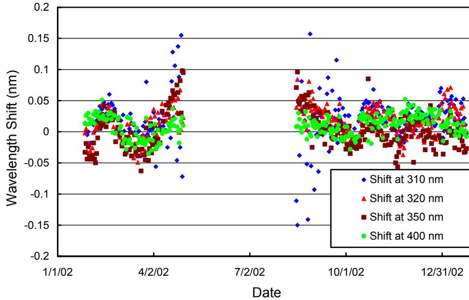
**Figure 5.1.9.** Check of the wavelength accuracy of the final data at four wavelengths by means of Fraunhofer correlation. The noontime measurement has been evaluated for each day of the season. No correlation data is available during the polar night.
