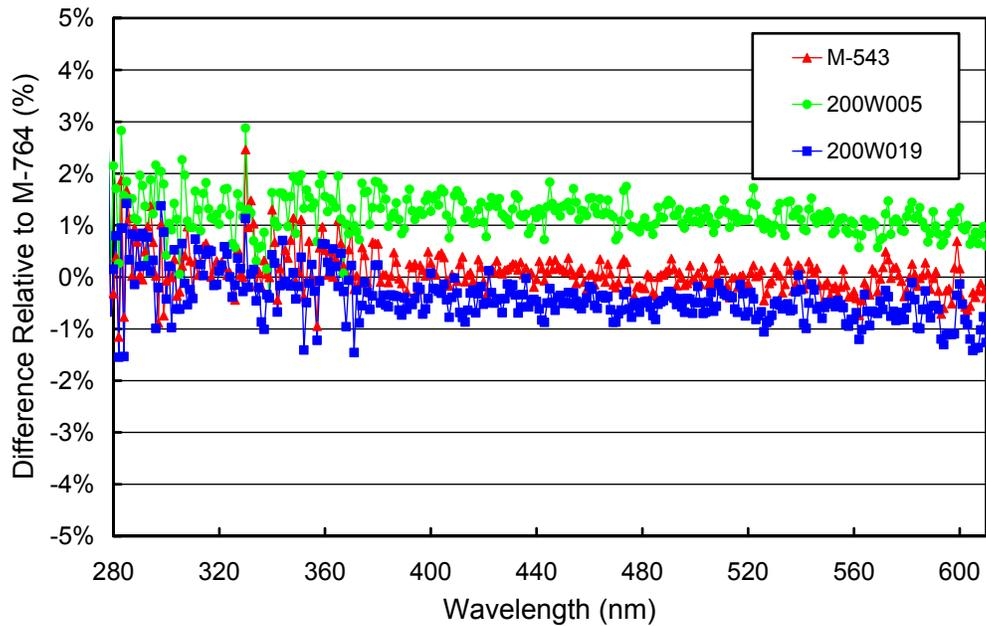
**Figure 5.1.3.** Comparison of McMurdo lamps M-543, 200W005, and 200W019 with the BSI traveling standard M-764 at the end of the season (1/23/03-1/24/03).
