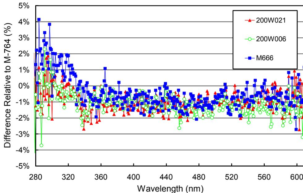
**Figure 5.3.1.** Comparison of South Pole lamps 200W006, 200W021, and M-666 with the BSI traveling standard M-764 at the start of the season on 1/18/01.
