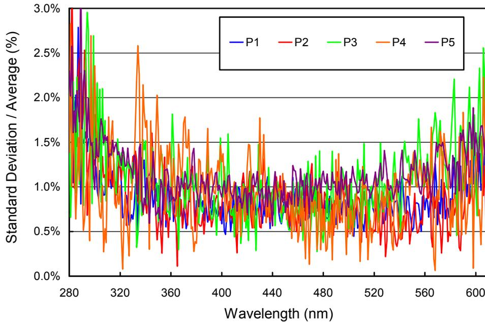
Figure 5.3.5. Ratio of standard deviation and average calculated from the absolute calibration scans measured during the South Pole 2001/02 season.
