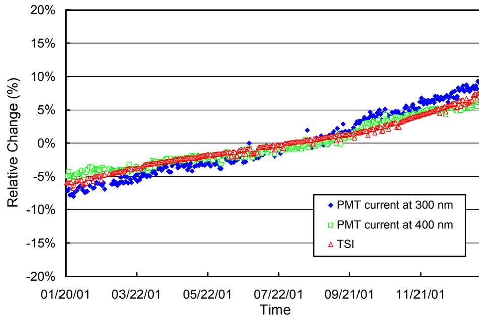
**Figure 5.3.3.** Time-series of PMT current at 300 and 400 nm, and TSI signal during measurements of the internal irradiance standard performed during the South Pole 2001/02 season. The data are normalized to the average of the whole period.
