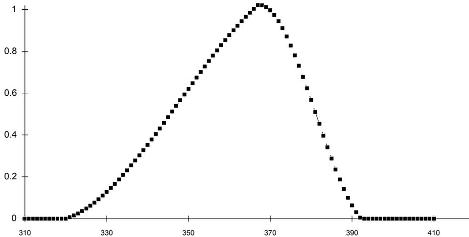
**Figure 2.6.** *Spectral response of the TSI sensor (typical).*
