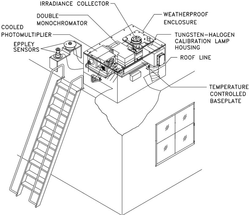
Figure 2.3. The spectroradiometer shown in a typical installation.
