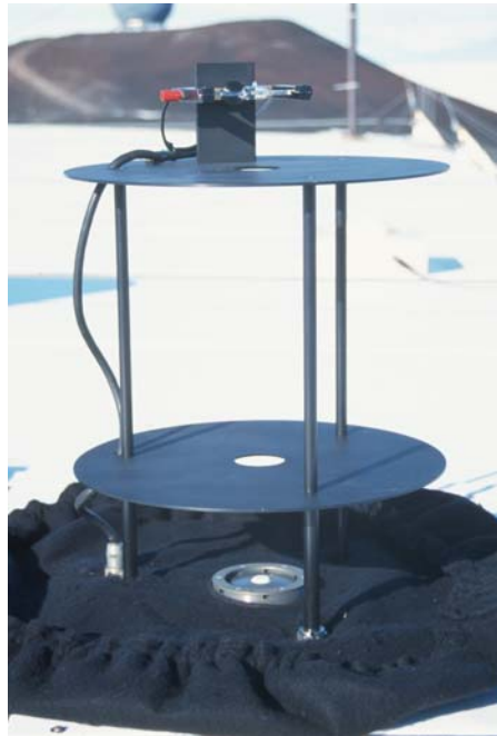
Figure 2.7. Calibration stand with the 200-Watt lamp mounted on top of the SUV-100. The lamp power is connected to the roofbox immediately below the fixture. Baffles limit stray light. During operation, an internally-blackened barrel covers this fixture.
