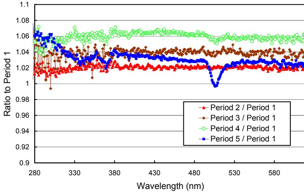
**Figure 5.3.6.** Ratios of the irradiance assigned to the internal lamp in Periods 2 – 4, relative to Period 1.
