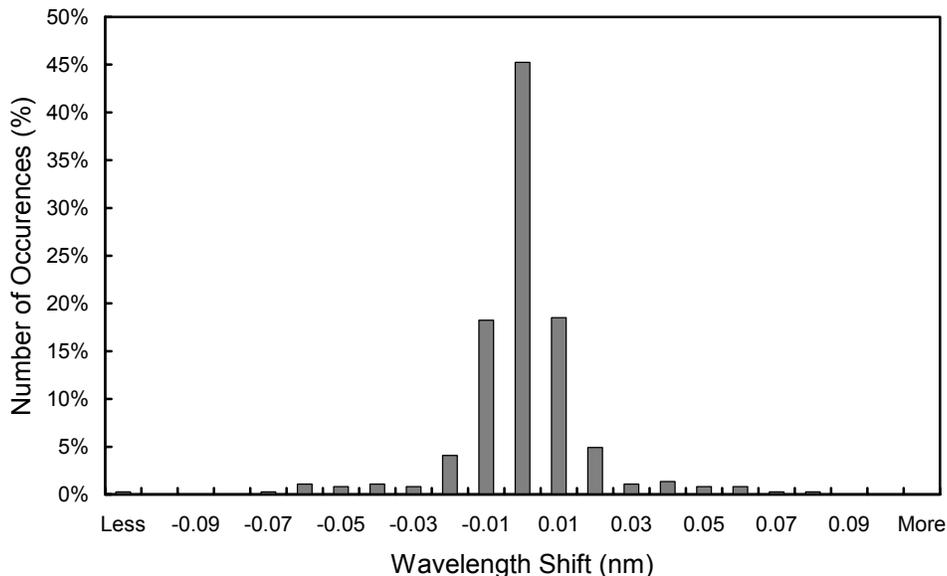
**Figure 5.3.8.** Differences in the measured position of the 296.73 nm mercury line between consecutive wavelength scans. The x-labels give the center wavelength shift for each column. The 0-nm histogram column covers the range -0.005 to +0.005 nm. “Less” means shifts smaller than -0.105 nm; “more” means shifts larger than 0.105 nm.
