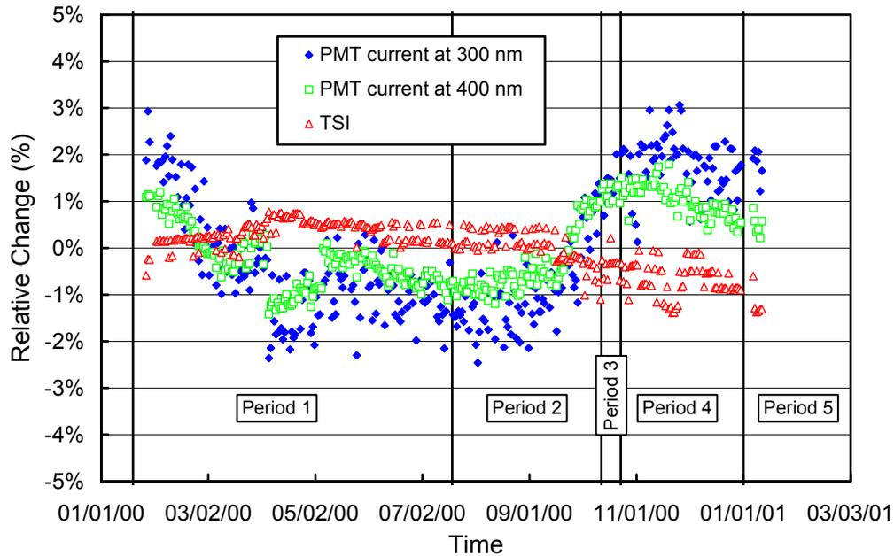
**Figure 5.3.3.** Time-series of PMT current at 300 and 400 nm, and TSI signal during measurements of the internal irradiance standard performed during the South Pole 2000/01 season. The data are normalized to the average of the whole period.
