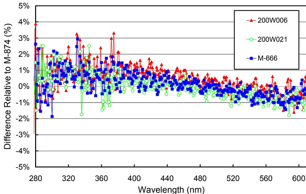
**Figure 5.3.1.** Comparison of South Pole lamps 200W006, 200W021, and M-666 with the BSI traveling standard M-874 at the start of the season on 1/25/00.
