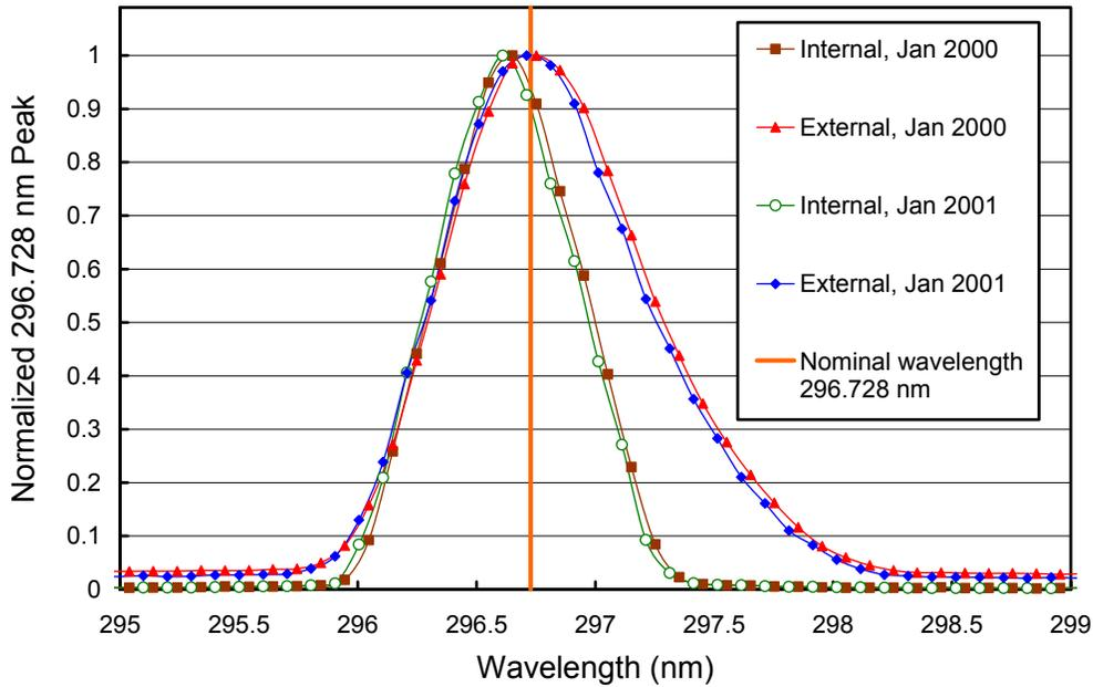
**Figure 5.3.11.** The 296.73 mercury line as registered by the PMT from external and internal sources. The wavelength scale is the same as applied for solar measurements, i.e., it is based on a combination of internal scans and the Fraunhofer-correlation method.
