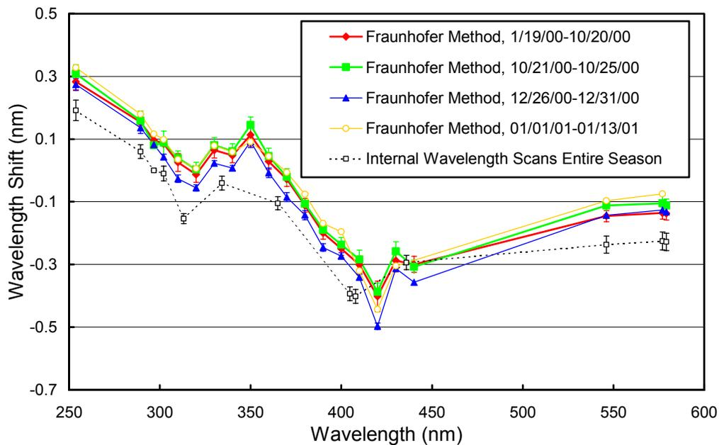
**Figure 5.3.9.** Monochromator non-linearity functions for the South Pole 2000/01 season. Thick lines: Correction functions calculated with the Fraunhofer-correlation method, applied to correct the South Pole Volume 10 data. Thin broken line: Correction function calculated with the method that was historically applied. The error bars show the  $1\sigma$  standard deviation of the wavelength shifts.
