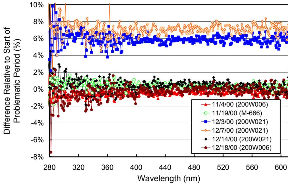
**Figure 5.3.4.** Comparison of absolute calibrations at South Pole performed between 11/4/00 and 12/18/00.
