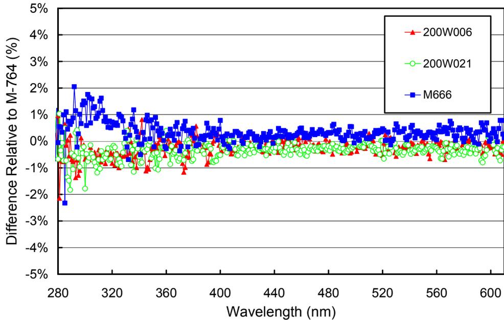
**Figure 5.3.2.** Comparison of South Pole lamps 200W006, 200W021, M-666 with the BSI traveling standard M-874 at the end of the season on 1/12/01.
