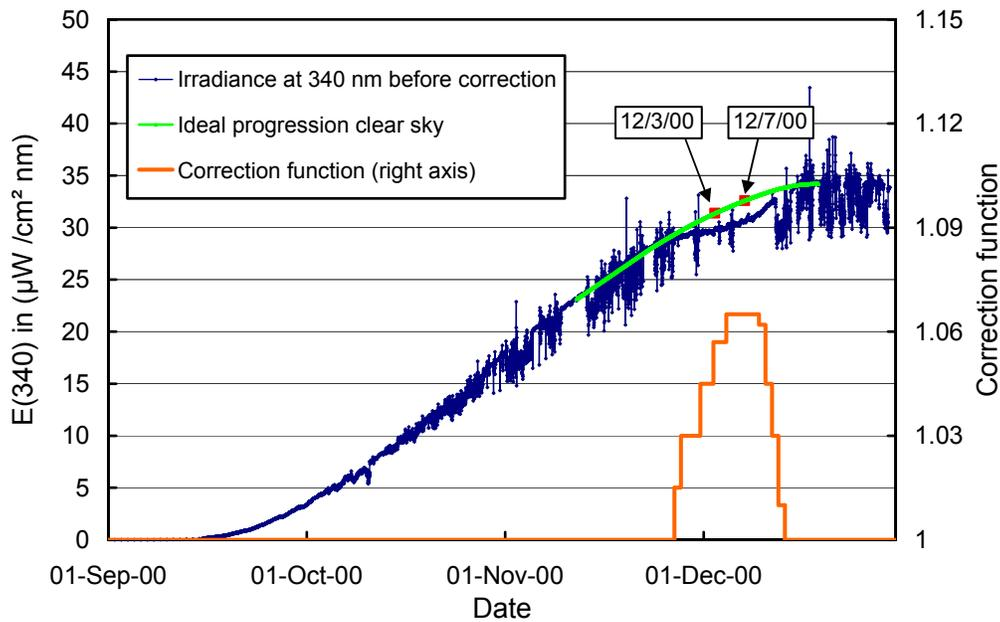
**Figure 5.3.5.** Effect of the ice build-up underneath the collector on solar irradiance at 340 nm.
