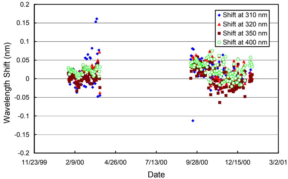
**Figure 5.3.10.** Wavelength accuracy check of the final data at four wavelengths by means of Fraunhofer correlation. The noontime measurement has been evaluated for each day of the season. No data exist during polar night.
