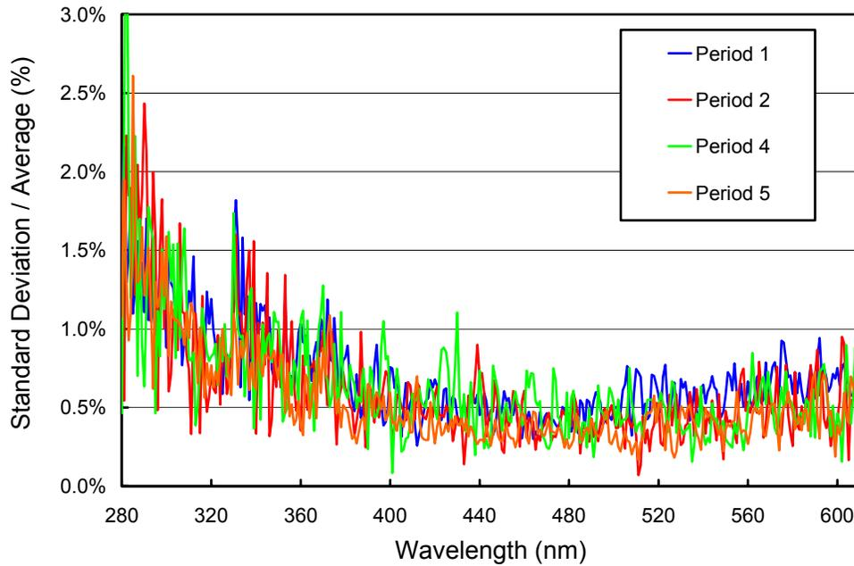
**Figure 5.3.7.** Ratio of standard deviation and average calculated from the absolute calibration scans measured during the South Pole 2000/01 season.
