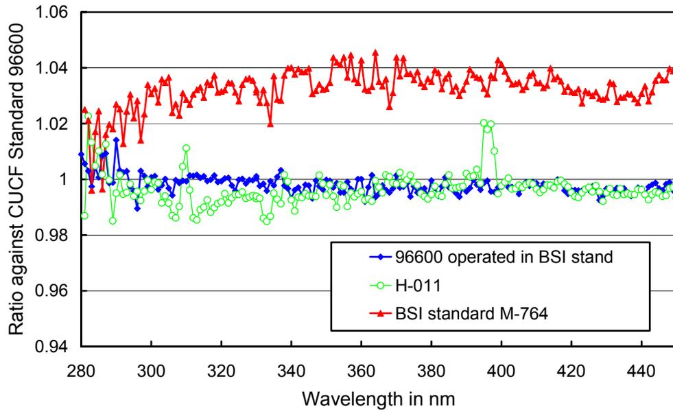
**Figure 5.2.** Results of the CUCF audit in October 2000. See text for details. The reference is a scan of CUCF standard 96600, mounted in CUCF field calibrator.
