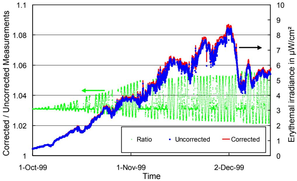
**Figure 5.7.** Comparison of corrected and uncorrected erythemal UV measurements at the South Pole, fall 1999.
