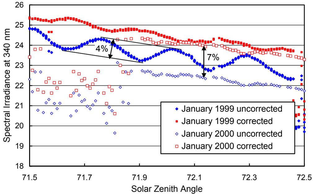
**Figure 5.8.** Comparison of cosine-corrected and cosine-uncorrected spectral irradiance at 340 nm, measured at the South Pole in 1999 (Volume 9, before collector modification) and 2000 (Volume 10, after collector modification).
