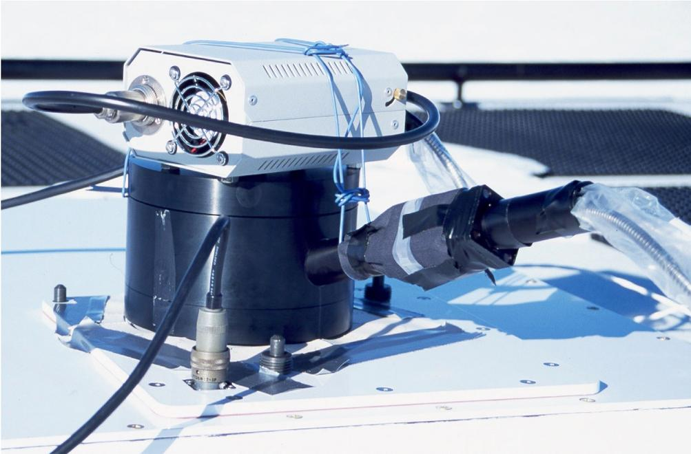
**Figure 5.5.** Apparatus for characterizing the angular response of SUV-100 spectroradiometer in operation at the South Pole. The white box on top is a light source, which is coupled via an optical fiber bundle and a baffled tube into the black cylinder shown in the center of the picture. The cylinder has precisely machined openings at 0°, 30°, 45°, 60°, and 70° zenith angles, and can be rotated to arbitrary azimuth angles.
