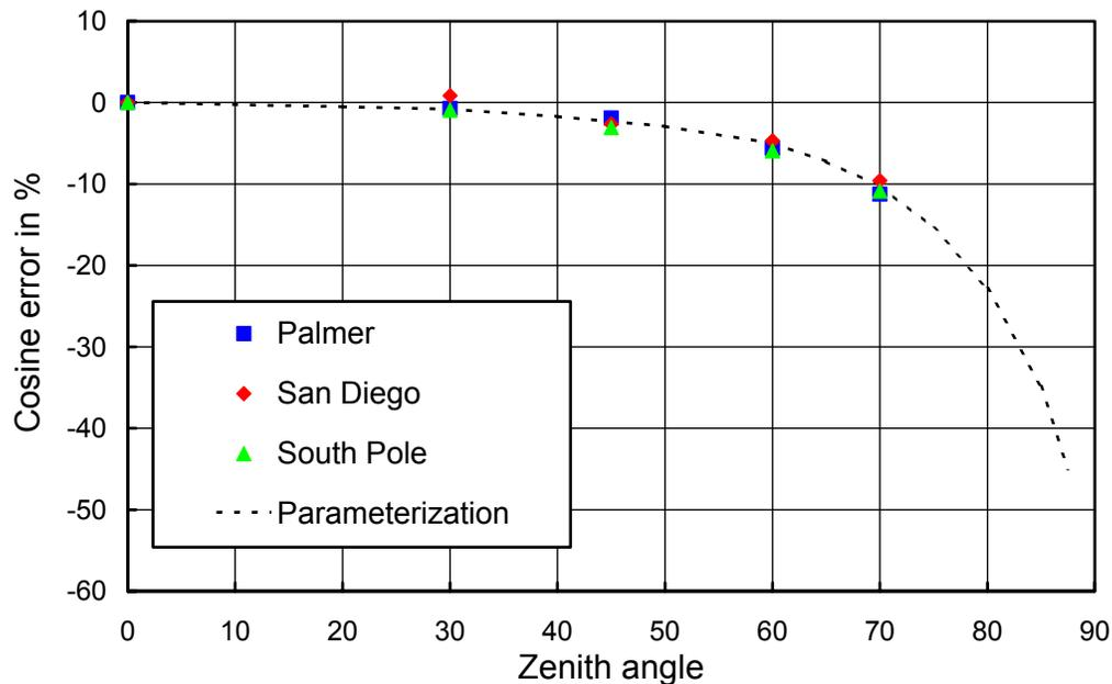
**Figure 5.6.** Cosine error of SUV-100 spectroradiometers after modification of the collector. The symbols represent measurements with the cosine test apparatus shown in Figure 5.5.
