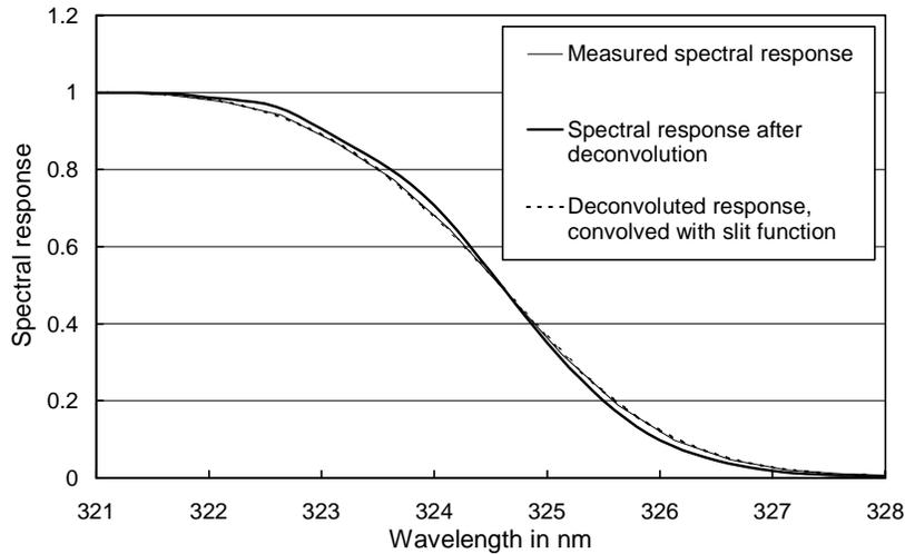
Figure 1: Comparison of measured (thin line) and deconvolved (thick line) spectral response of the 320 nm channel of GUV S/N 29236. The data set indicated by the broken line was calculated by convolving the deconvolved response  $R_D(\lambda)$  with the slit function of the of the test apparatus.
