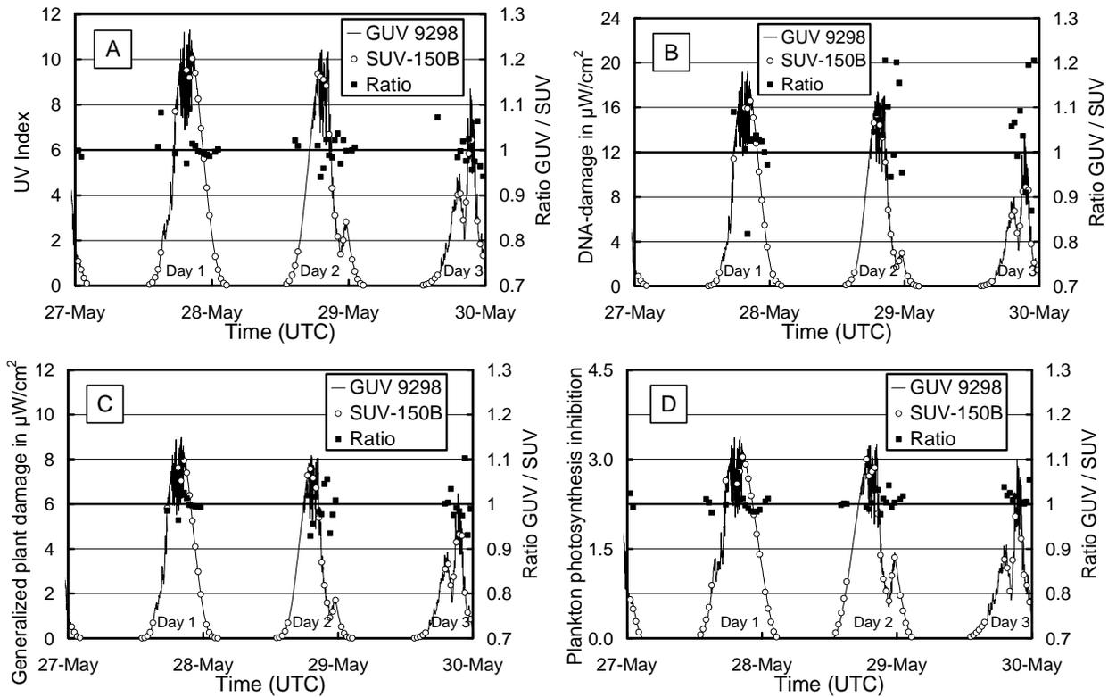
Figure 6: Comparison of four different data products measured by GUV S/N 9298 and SUV-150B at San Diego between May 27 and May 30, 2003. The ratios of GUV and SUV measurements are shown for periods when radiation levels exceed 10% of the maximum levels observed at noon. Panel A: UV Index; Panel B: DNA-damaging radiation, Panel C: Generalized plant response; Panel D: Inhibition of photosynthesis in Antarctic phytoplankton.
