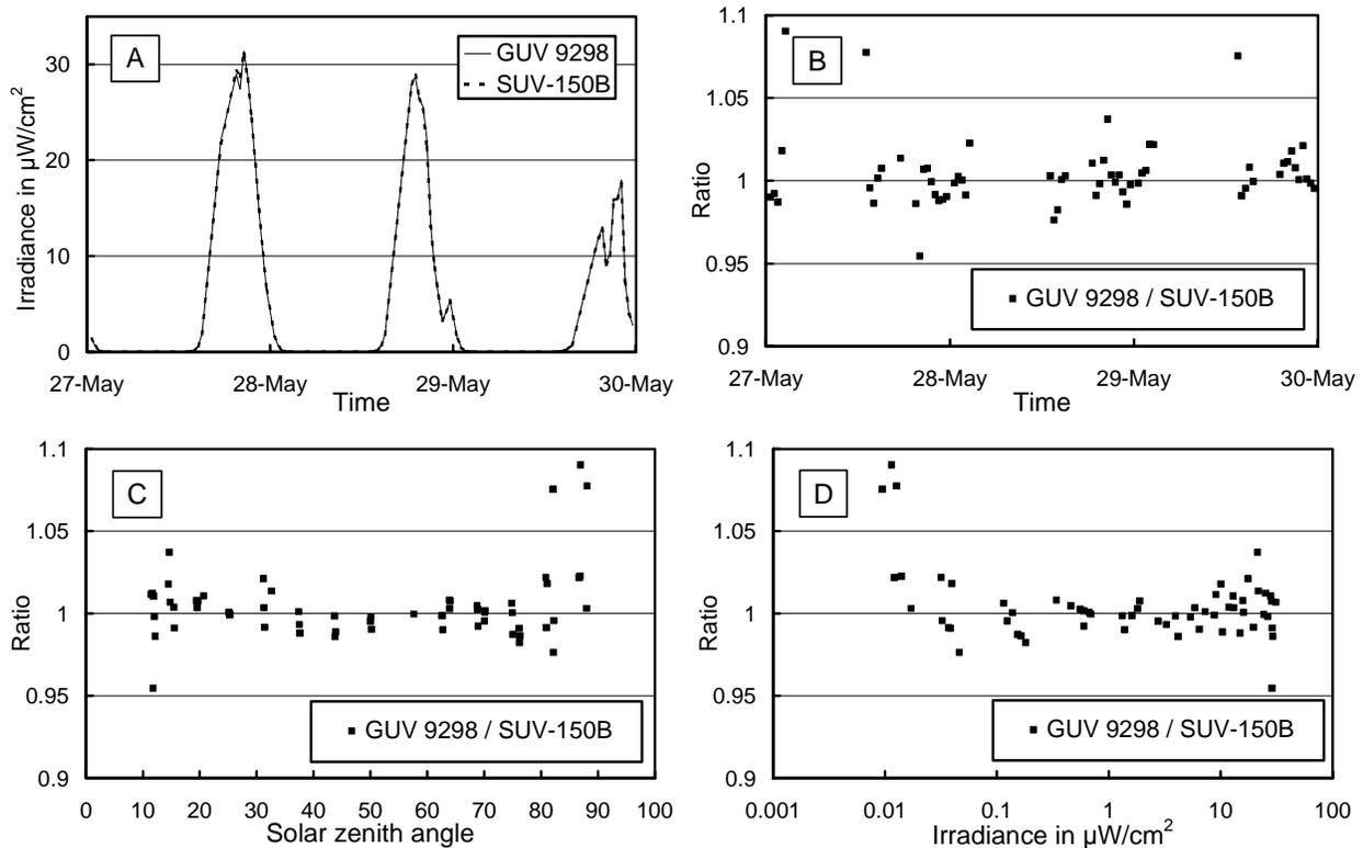
Figure 3: Comparison of measurements from the 305 nm channel of GUV S/N 9298 and the SUV-150B. The calibration factor  $k_{305}$  of the GUV was calculated by regressing GUV measurements against the weighted SUV-150B spectra. Panel A: Irradiance measured by GUV and SUV as a function of time. Panel B: Ratio GUV / SUV as a function of time. Panel C: Ratio GUV / SUV as a function of solar zenith angle. Panel D: Ratio GUV / SUV as a function of spectral irradiance (Note the logarithmic x-axis).
