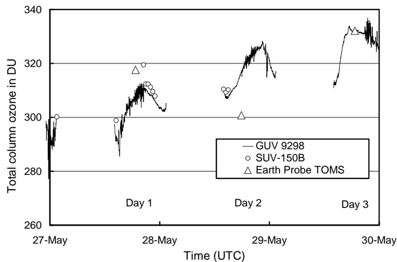
Figure 7: Comparison of total column ozone measured by GUV S/N 9298, SUV-150B and Earth Probe TOMS satellite at San Diego between May 27 and May 30, 2003.
