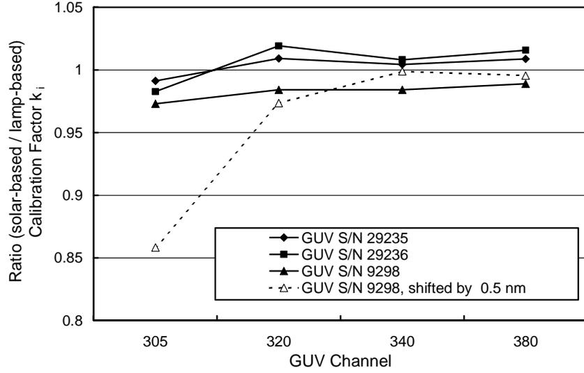
Figure 5: Comparison of solar- and lamp-based calibration factors  $k_i$  for three different GUV radiometers. The calibration factors marked with solid symbols were calculated with the measured response functions of the radiometers. The data set marked with open triangles was calculated with the shifted response functions of GUV S/N 9298 (shift = 0.5 nm) to investigate the effect of wavelength errors on the resulting calibration factors.
