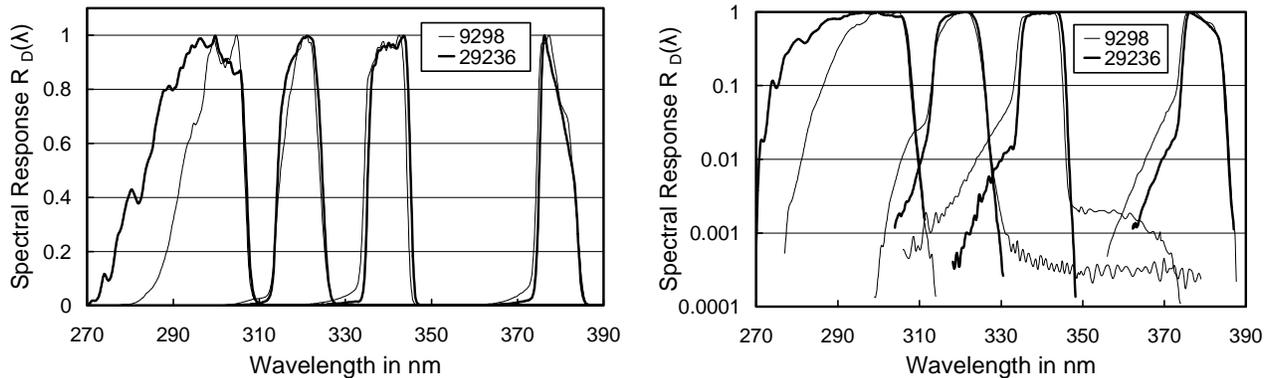
Figure 2: Spectral response functions  $R_D(\lambda)$  of the 305, 320, 340, and 380 nm channels of two GUV radiometers (S/N 9298 and 29236) in linear (left panel) and logarithmic (right panel) presentation.
