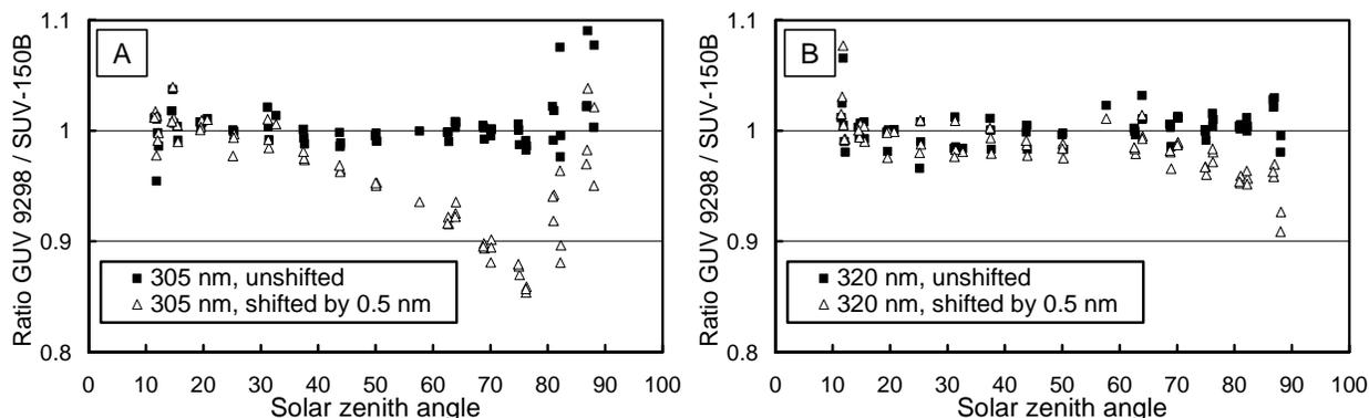
Figure 4: Comparison of measurements from the 305 and 320 nm channels of GUV S/N 9298 and the SUV-150B using either the measured, unshifted GUV response functions  $R_{D_i}(\lambda)$  (solid squares), or response functions constructed by shifting  $R_{D_i}(\lambda)$  by 0.5 nm (open triangles). Panel A: Comparison for the GUV 305 nm channel (the unshifted data set is identical with the one shown in Figure 3C). Panel B: Comparison for the GUV 320 nm channel.
