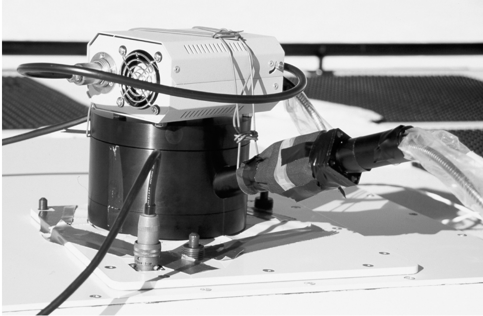
Figure 2: Apparatus for characterizing the angular response of SUV-100 spectroradiometer in operation at the South Pole. The white box on top is a light source, which is coupled via an optical fiber bundle and a baffled tube into the black cylinder shown in the center of the picture. The cylinder has precisely machined openings at 0°, 30°, 45°, 60°, and 70° zenith angles, and can be rotated to arbitrary azimuth angles.
