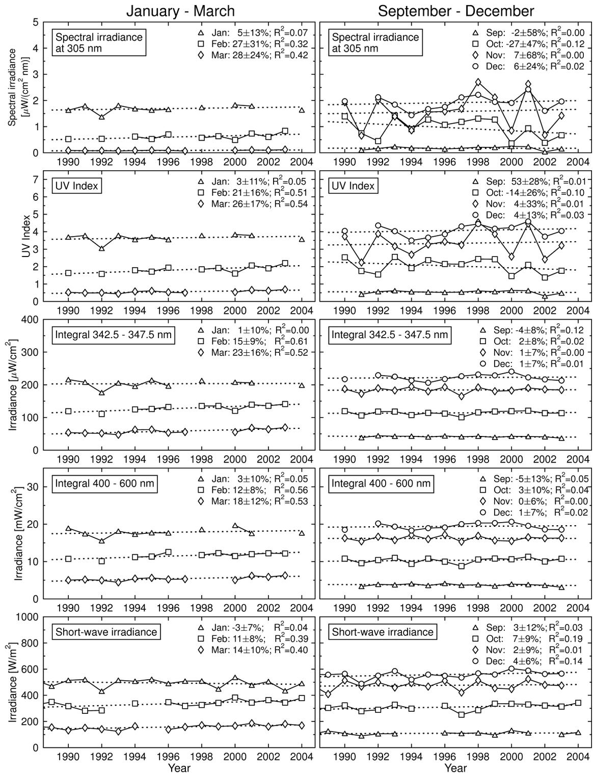
**Figure 2:** Time series of average noon-time measurements for months of January – March (left column) and September – December (right column) and five data products, indicated in the top left corner of each plot. Dashed lines are trend lines determined by linear regression. Trend per decade relative to 1990,  $2\sigma$ -uncertainty of trend, and regression coefficient  $R^2$  are also indicated in the legend of each plot.
