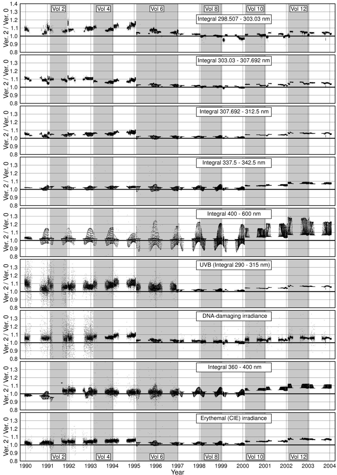
**Figure 1.** Ratio of Version 2 to Version 0 for the integrals 298.507 – 303.03 nm, 303.03 – 307.692 nm, 307.692 – 312.5 nm, 337.5 – 342.5 nm, 400 – 600 nm, 290 – 315 nm, and 360 – 400 nm; as well as DNA damaging and erythema irradiance. Gray shading marks data that are part of even numbered Volumes as indicated on the top and bottom of the graph.
