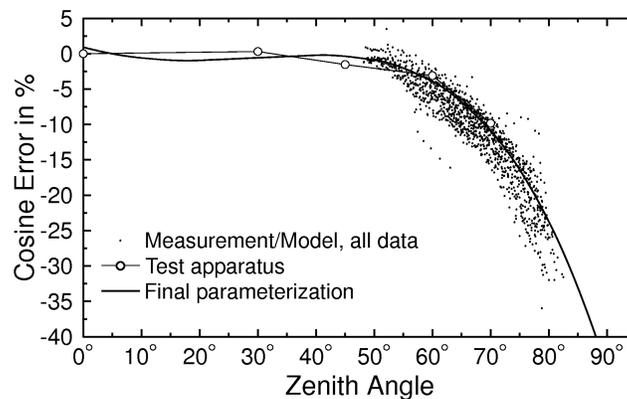
**Figure 1.** Cosine error of the SUV-100 spectroradiometer at Barrow determined from a comparison of measured and modeled spectral irradiance at 600 nm and measurements with the test apparatus. Data is from Volume 14, covering the years 2004-2005. The cosine error of other volumes may be different.
